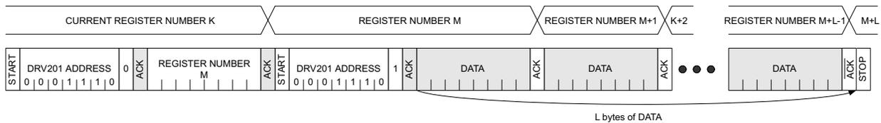
Figure 9. Sequential Read from a Defined Location
