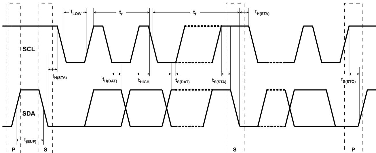
**Figure 13. I<sup>2</sup>C Data Transmission Protocol**
