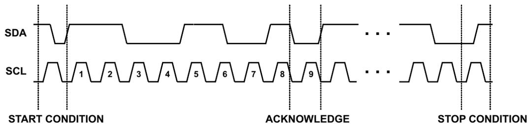
**Figure 12. I<sup>2</sup>C Start/Stop/Acknowledge Protocol**
