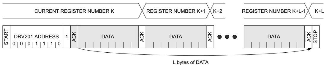
Figure 11. Sequential Read Starting from a Current Location
