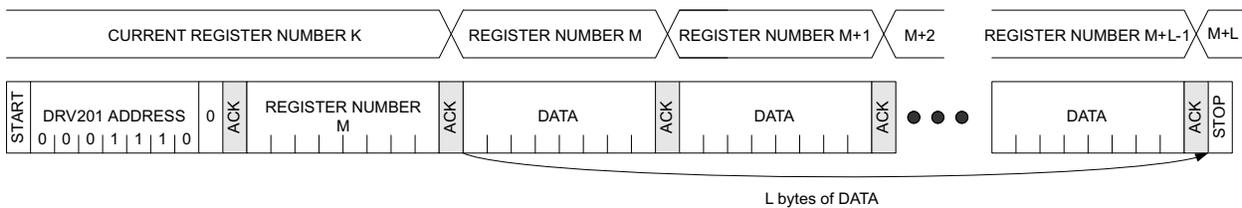
Figure 10. Sequential Write
