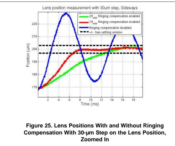
Figure 25. Lens Positions With and Without Ringing Compensation With 30- $\mu$ m Step on the Lens Position, Zoomed In
