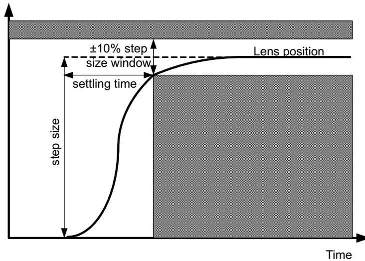
Figure 21. Lens Settling Time and Settling Window
