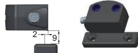
Lateral actuation only from the shown sensor side.
