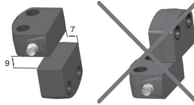
Lateral actuation only from the shown sensor side.
