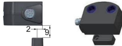
Lateral actuation only from the shown sensor side.
