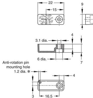
\* D41D-A3 mounting hole is fixed in place with an M3 screw. The actuator can be prevented from twisting caused by screw tightening torque during installation by passing a pin up to 1.1 mm in size through the hole in the rear section of the D41D-A3.
