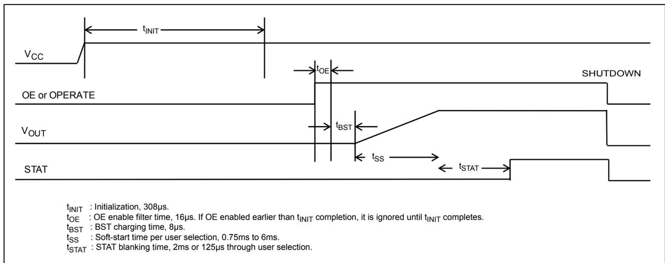
Figure 1. Startup Timing
