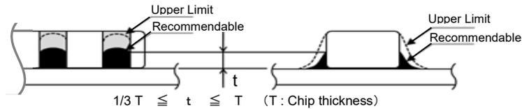
Accordingly increasing the solder volume, the mechanical stress to product is also increased. Excessive solder volume may cause the failure of mechanical or electrical performance.
