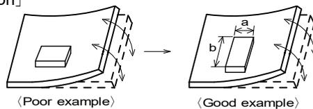
Products shall be location the sideways Direction (Length : a<b) to the machanical Stress.
