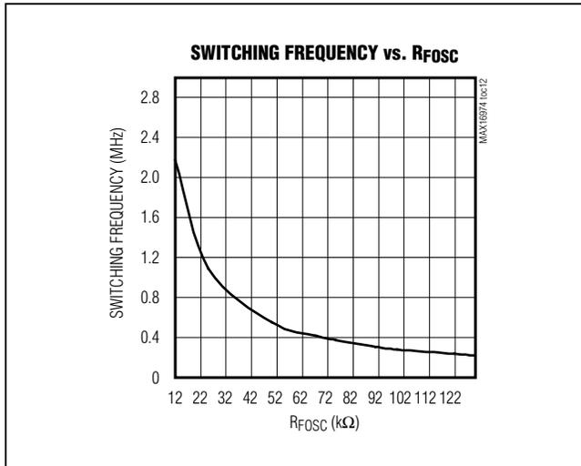
Figure 4. Switching Frequency vs. R<sub>FOSC</sub>
