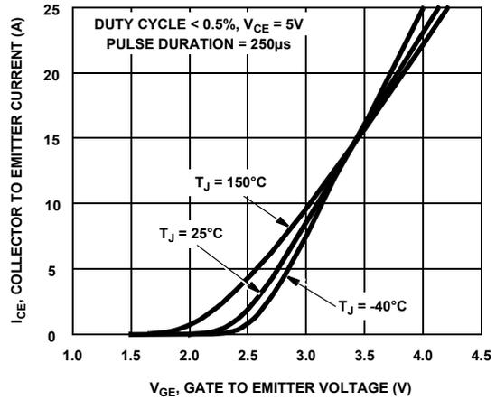
Figure 8. Transfer Characteristics
