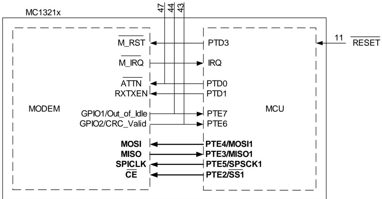
Figure 4. MC1321x Internal Interconnects Highlighting SPI Bus
