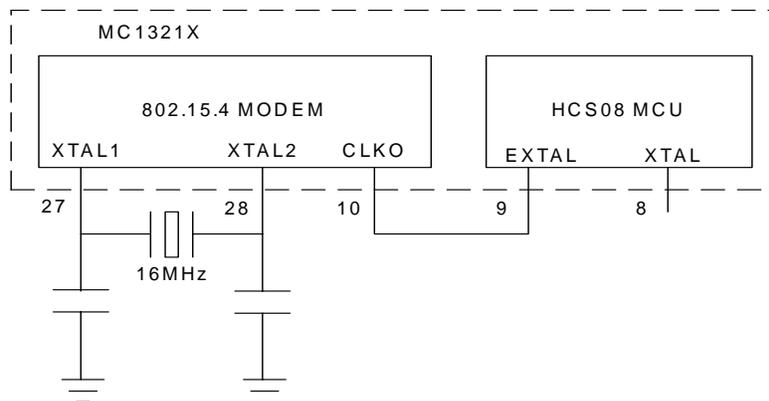
Figure 2. MC1321x Single Crystal System Clock Structure
