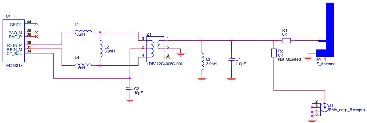
Figure 35. RF Single Port Application with an F-Antenna
