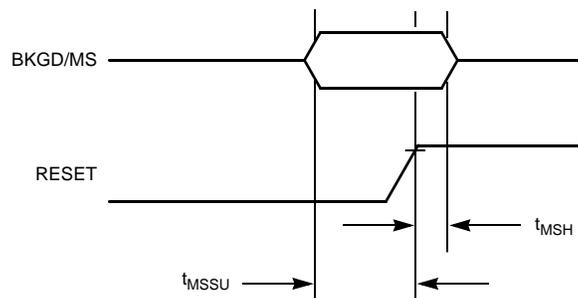
**Figure 29. Control Active Background Debug Mode Latch Timing**
