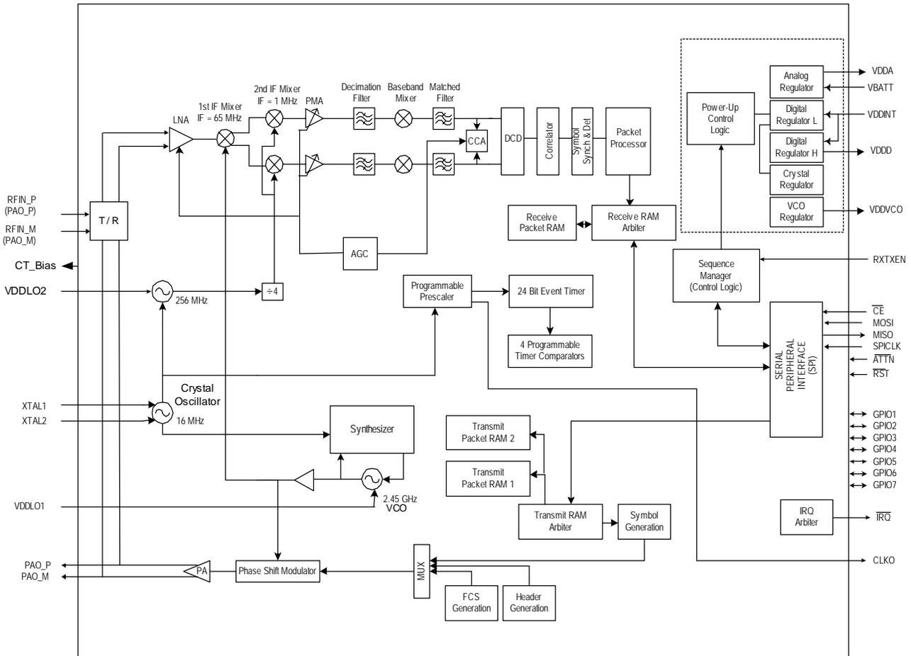
Figure 6. 802.15.4 Modem Block Diagram
