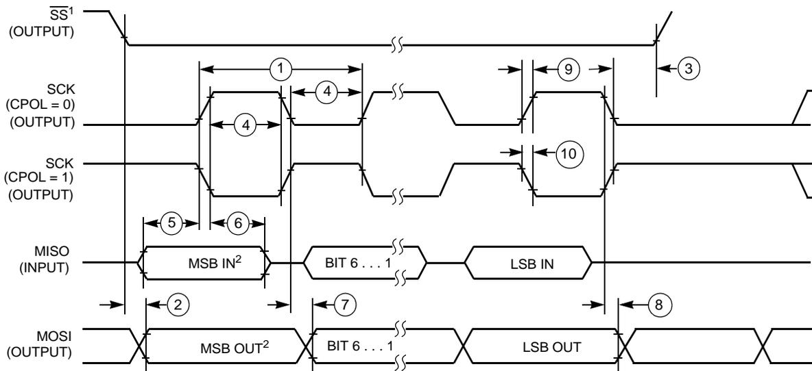
Figure 33. SPI Master Timing (CPHA = 0)
