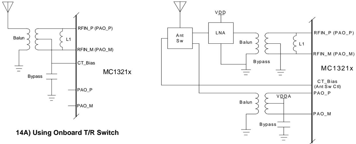
14A) Using Onboard T/R Switch
