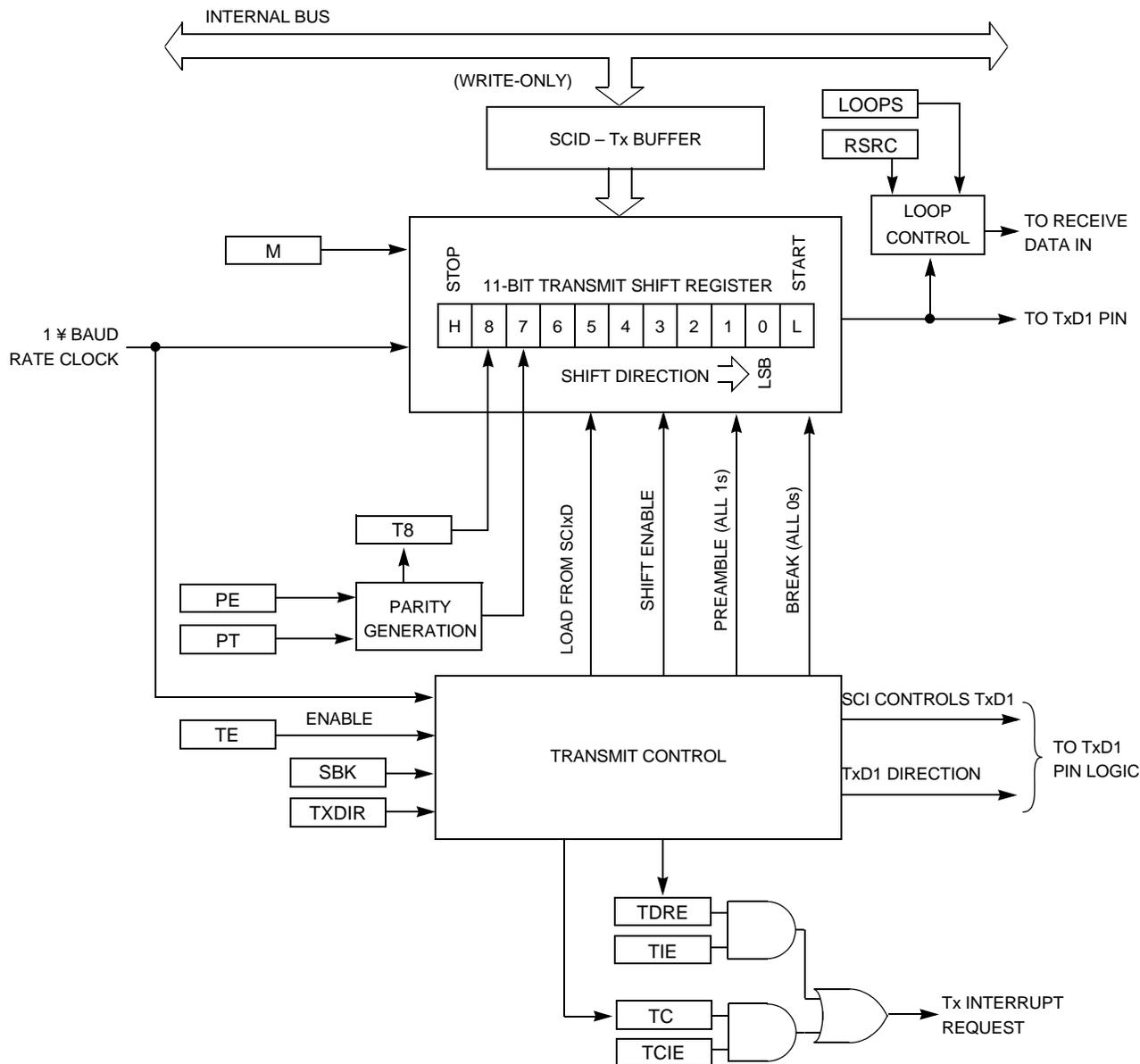
Figure 22. SCI Transmitter
