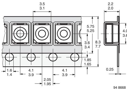
Fig. 7 - Tape Dimensions in mm for PLCC-2
