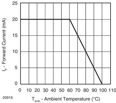
Fig. 1 - Forward Current vs. Ambient Temperature for GaN
