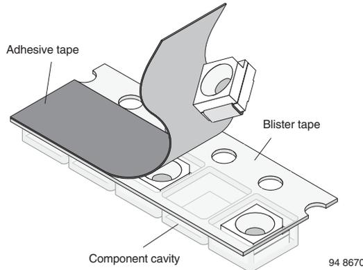
**REEL PACKAGE DIMENSION IN MILLIMETERS FOR SMD LEDs, TAPE OPTION GS18 (= 8000 PCS) PREFERRED**
