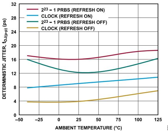
Figure 29. Deterministic Jitter,  $t_{DJ(p-p)}$  vs. Ambient Temperature
