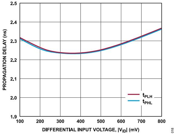
Figure 21. Propagation Delay vs. Differential Input Voltage,  $|V_{ID}|$
