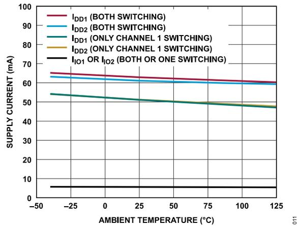
Figure 14. Supply Current vs. Ambient Temperature, ADN4621
