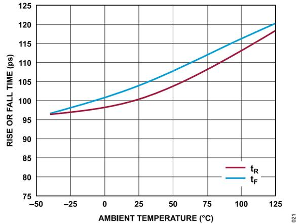
Figure 24. Rise or Fall Time vs. Ambient Temperature
