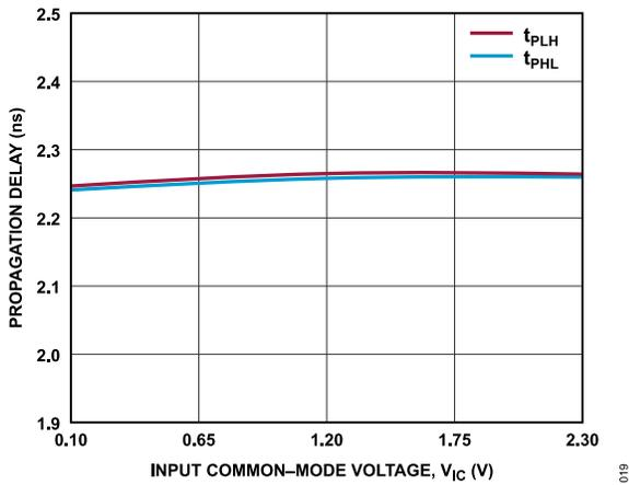
Figure 22. Propagation Delay vs. Input Common-Mode Voltage,  $V_{IC}$
