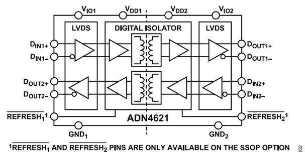
Figure 2. ADN4621 One Forward and One Reverse Channel
