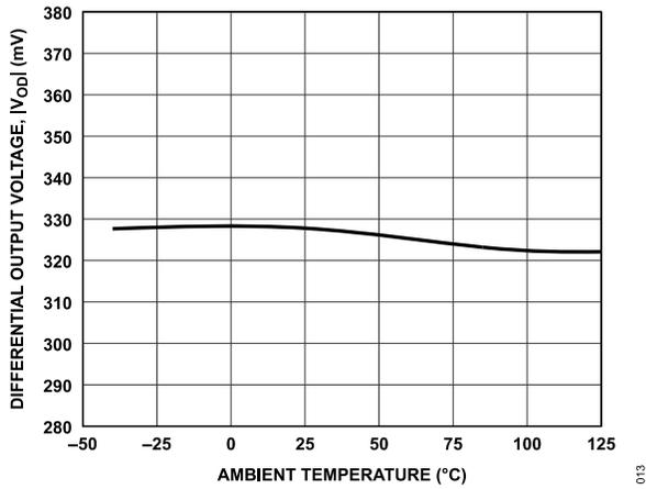
Figure 16. Differential Output Voltage,  $|V_{OD}|$  vs. Ambient Temperature
