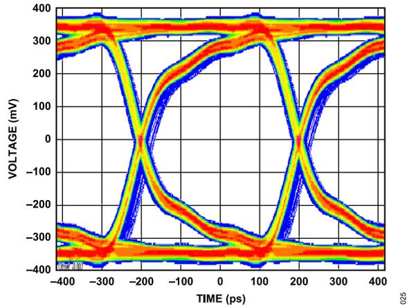
Figure 33. Eye Diagram for  $D_{OUT1\pm}$  at 1.25 GHz
