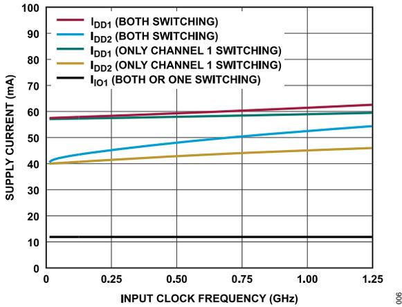
Figure 9. Supply Current vs. Input Clock Frequency, ADN4620
