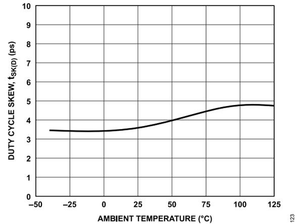
Figure 26. Duty Cycle Skew,  $t_{SK(D)}$  vs. Ambient Temperature
