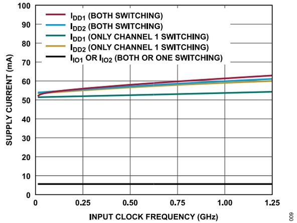
Figure 12. Supply Current vs. Input Clock Frequency, ADN4621
