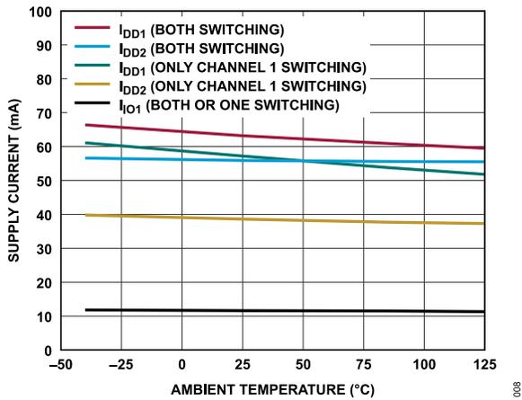
Figure 11. Supply Current vs. Ambient Temperature, ADN4620
