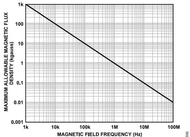
Figure 40. Maximum Allowable External Magnetic Flux Density
