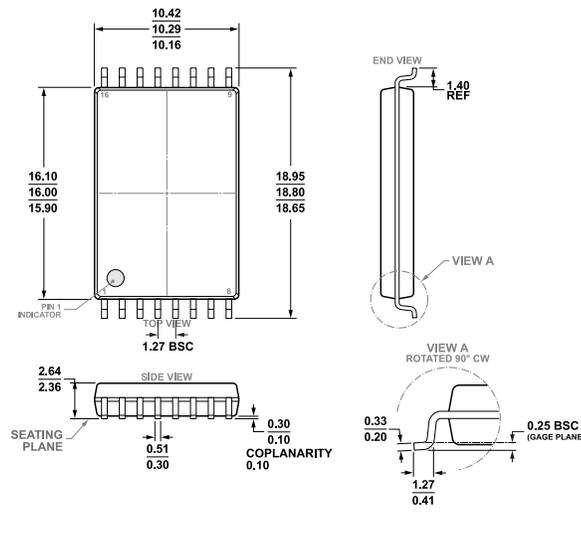
Figure 44. 16-Lead Standard Small Outline Package, with 15.1 mm Creepage [SOIC\_IC] Wide Body (RI-16-3)
