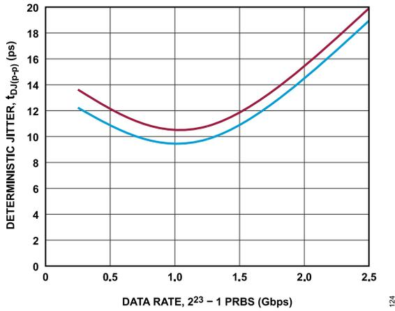
Figure 27. Deterministic Jitter,  $t_{DJ(p-p)}$  vs. Data Rate,  $2^{23} - 1$  PRBS
