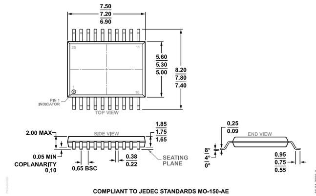
Figure 43. 20-Lead Shrink Small Outline Package [SSOP] (RS-20)
