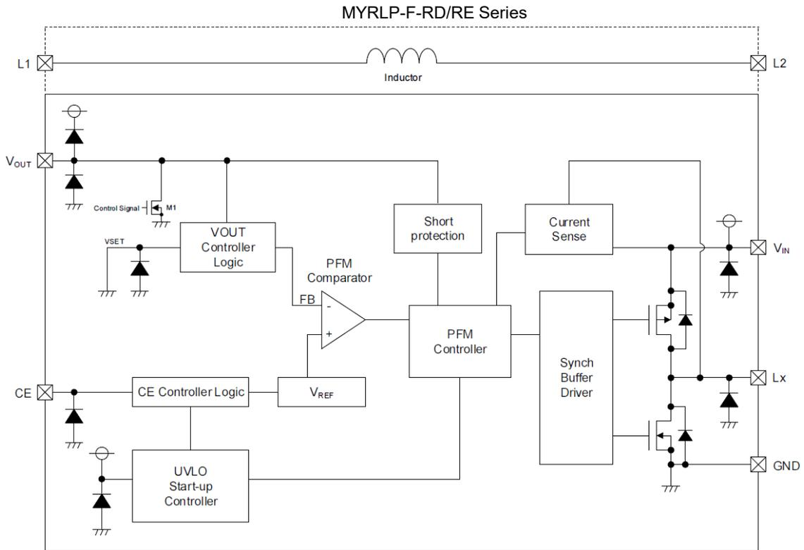
\* Diodes inside the circuits are ESD protection diodes and parasitic diodes.
