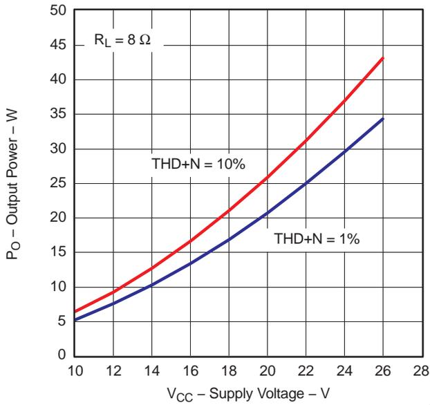
Figure 11. Output Power Vs. Supply Voltage (BTL)
