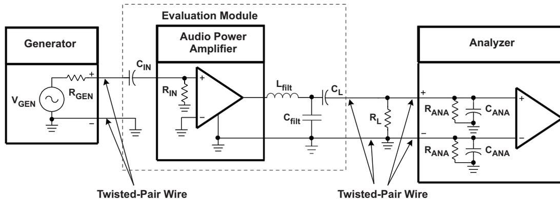
**Figure 20. SE Input—SE Output Measurement Circuit**
