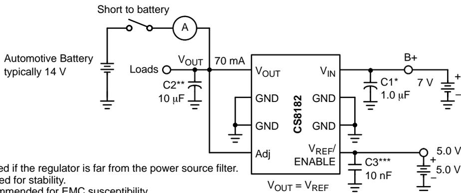
\* C1 is required if the regulator is far from the power source filter.
