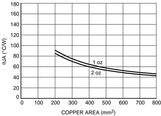
Figure 20. 5 Lead D<sup>2</sup>PAK Thermal Resistance
