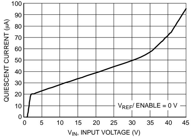
Figure 4. Quiescent Current vs. Input Voltage (Sleep Mode)
