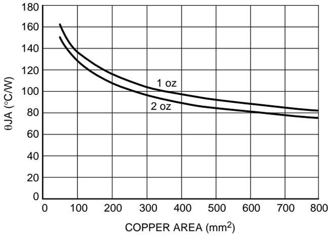
Figure 18. 8 Lead SOIC (Fused) Thermal Resistance
