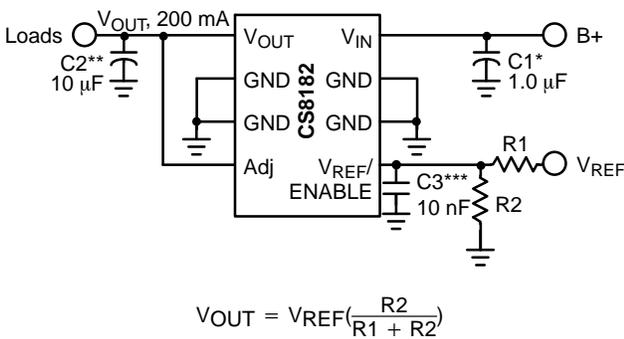
Figure 9. Tracking Regulator at Lower Voltages
