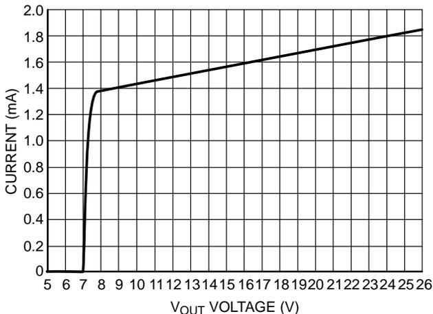
Figure 15. V<sub>OUT</sub> Short to Battery
