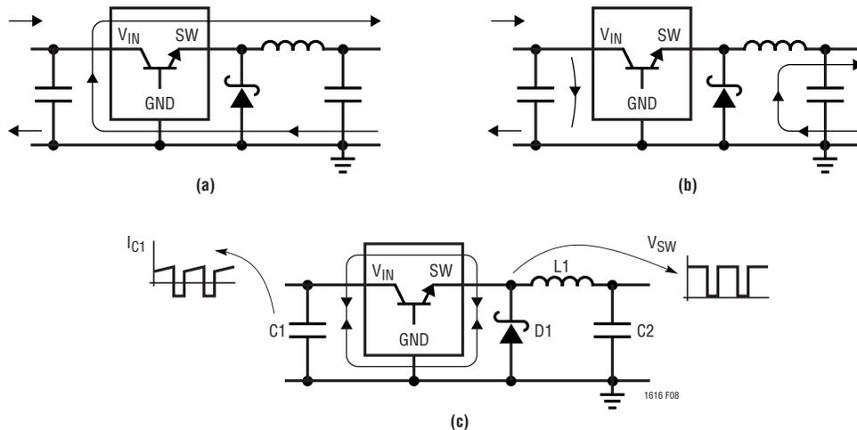
**Figure 8. Subtracting the Current When the Switch is On (a) from the Current When the Switch is Off (b) Reveals the Path of the High Frequency Switching Current (c). Keep This Loop Small. The Voltage on the SW and BOOST Nodes Will Also be Switched; Keep These Nodes as Small as Possible. Finally, Make Sure the Circuit is Shielded with a Local Ground Plane**
