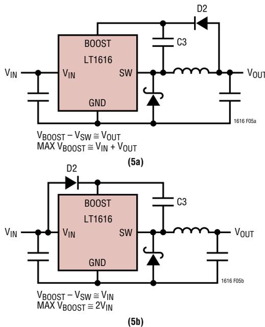
Figure 5. Two Circuits for Generating the Boost Voltage
