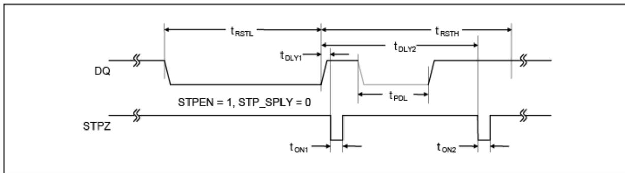
Figure 10. STPZ timing during the reset/presence detect cycle.
