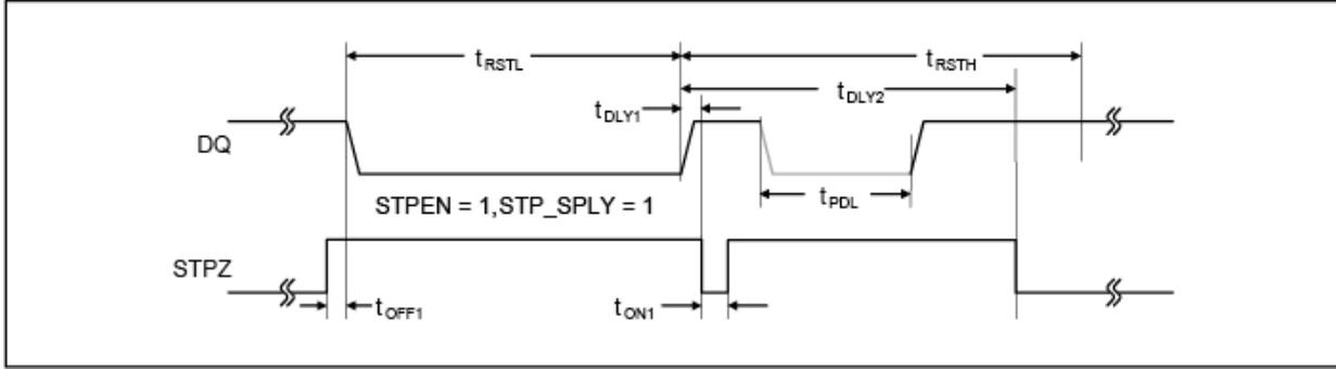
Figure 12. STPZ timing with power delivery during the reset/presence detect cycle.
