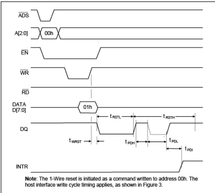
**Note:** The 1-Wire reset is initiated as a command written to address 00h. The host interface write cycle timing applies, as shown in Figure 3.
