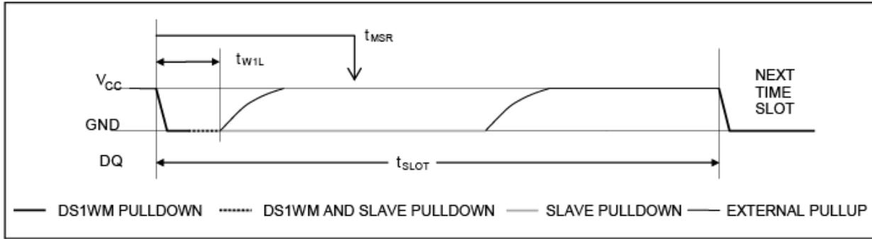
Figure 9. Read-data time slot.
