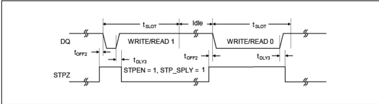
Figure 13. STPZ timing with power delivery during read/write time slots.
