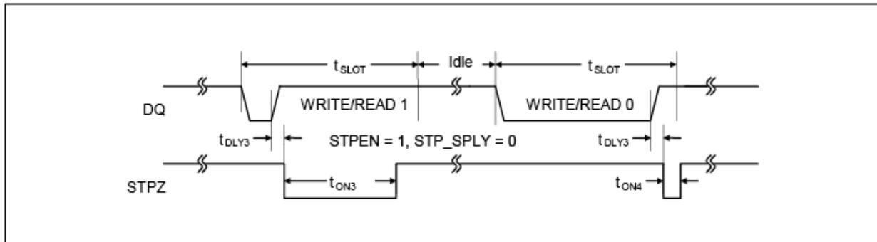
Figure 11. STPZ timing during read/write time slots.
