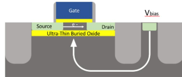
*Body Biasing: Faster when required and more energy efficient when performance isn't as critical*
