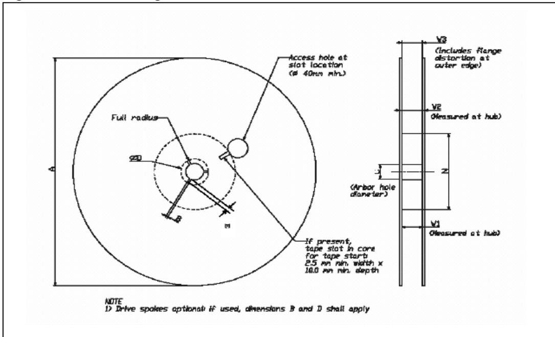
Table 27. Tape and reel dimensions for TFBGA25 (12 mm width)
