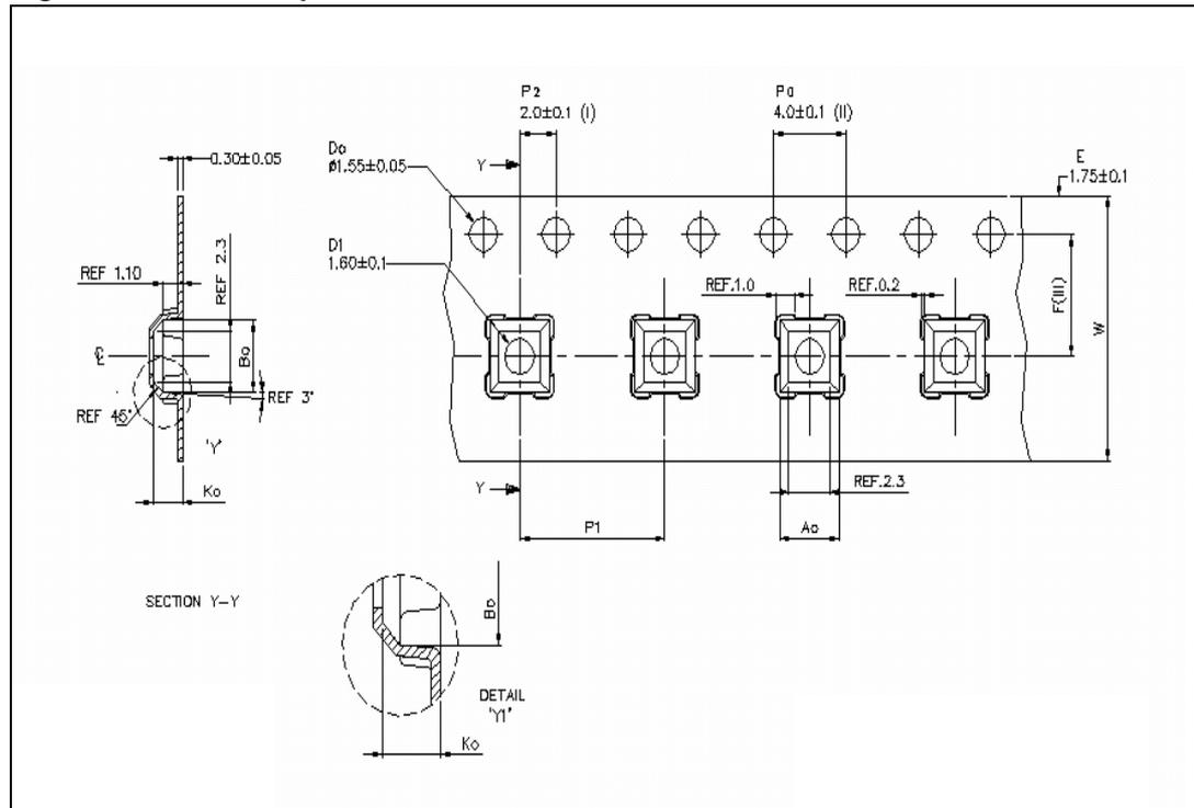
Table 26. Carrier tape mechanical data for TFBGA25
