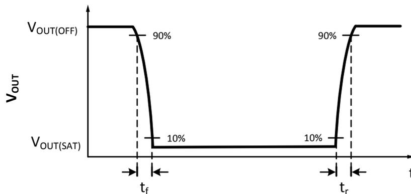
Figure 2: Definition of Output Rise and Fall Time
