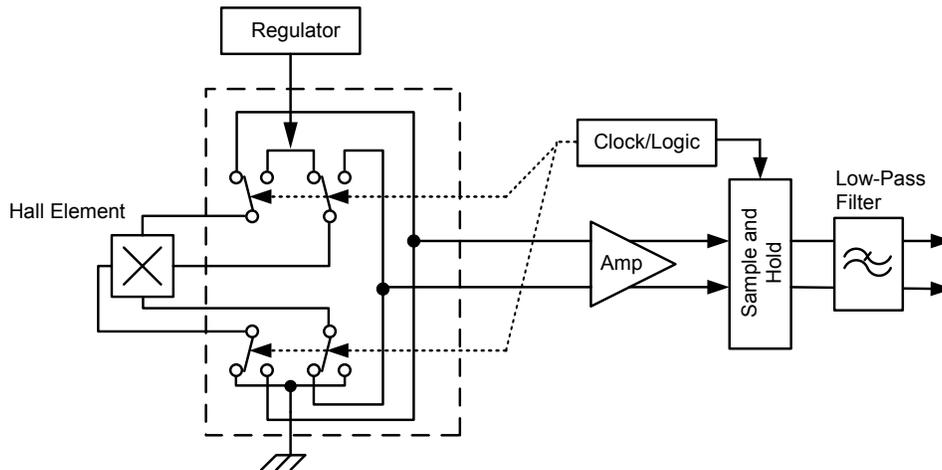
**Figure 8: Model of Chopper Stabilization Circuit
