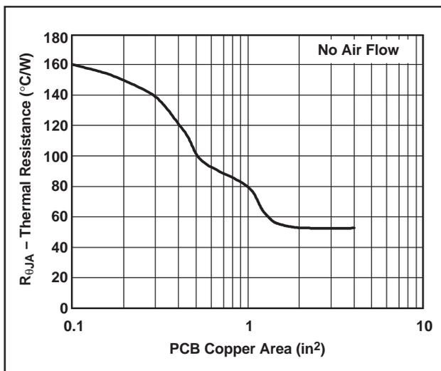
Figure 25. SOT223 Thermal Resistance vs PCB Copper Area
