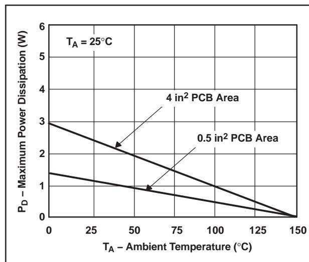
Figure 26. SOT223 Maximum Power Dissipation vs Ambient Temperature
