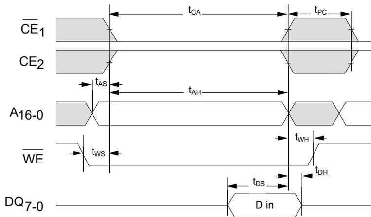
Figure 9. Write Cycle Timing 3 ( $\overline{CE1}$  LOW,  $\overline{CE2}$  HIGH) <sup>[11]</sup>
