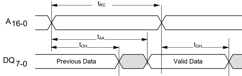
Figure 5. Read Cycle Timing 2 (Chip Enable Controlled)
