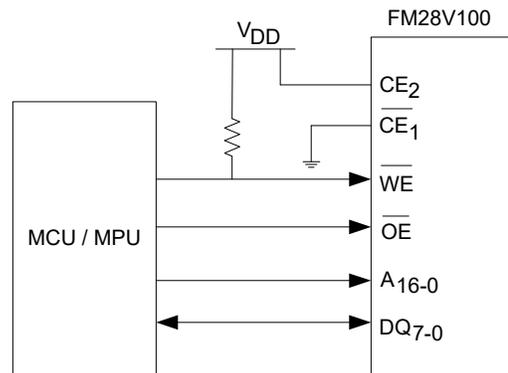
For applications that require the lowest power consumption, the chip enable signal should be active only during memory accesses. Due to the external pull-up resistor, some supply current will be drawn while  $\overline{CE}_1$  is LOW. When  $\overline{CE}_1$  is HIGH, the device draws no more than the maximum standby current  $I_{SB}$ .
