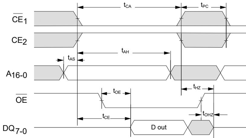
Figure 6. Page Mode Read Cycle Timing <sup>[10]</sup>
