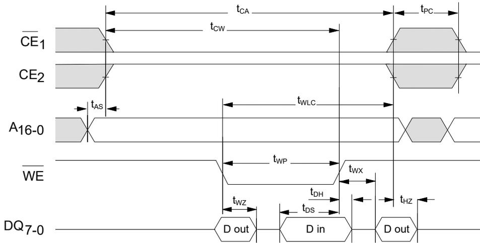
Figure 8. Write Cycle Timing 2 ( $\overline{CE}$  Controlled)
