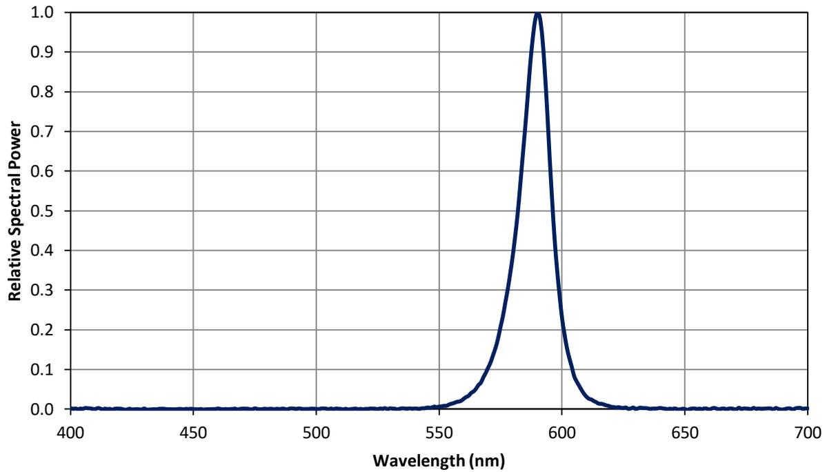
Figure 5: Relative spectral power vs. wavelength @ T<sub>c</sub> = 25°C.
