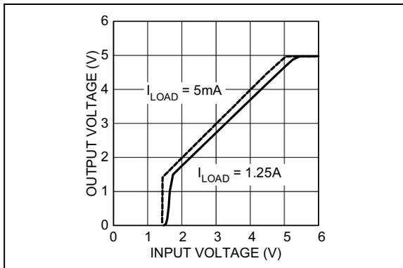
**FIGURE 2-3:** Dropout Characteristics.
