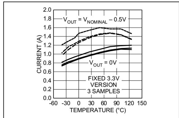
**FIGURE 2-11:** Short-Circuit and Maximum Current vs. Temperature.
