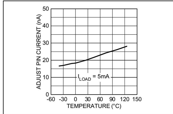
**FIGURE 2-16:** MIC2941A Adjust Pin Current vs. Temperature.
