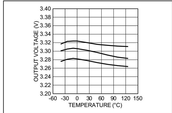
**FIGURE 2-10:** Fixed 3.3V Output Voltage vs. Temperature.
