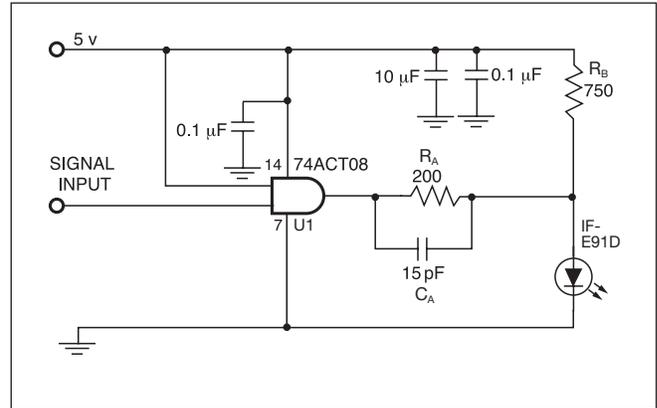
FIGURE 3. Test application circuit ( $I_F = 22\text{mA}$ ).
