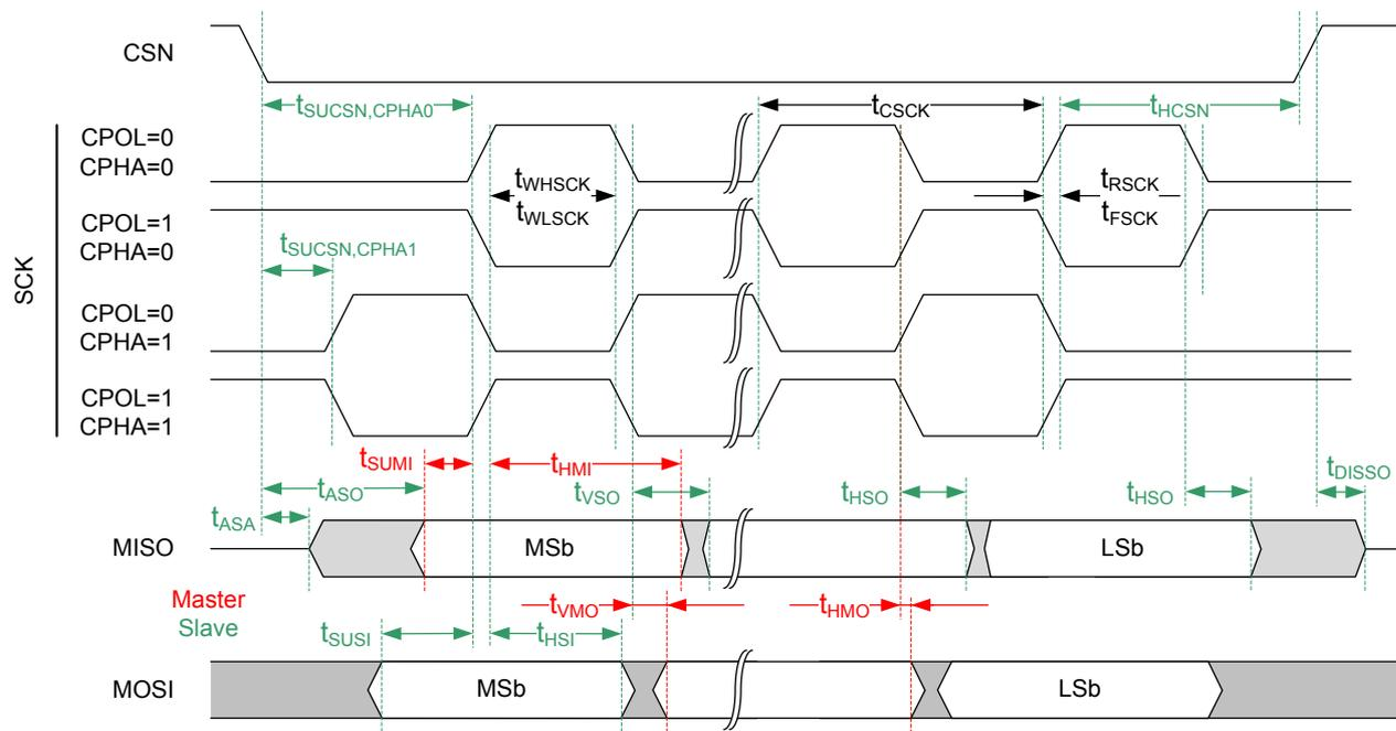
Figure 78: Common SPIM and SPI timing diagram
