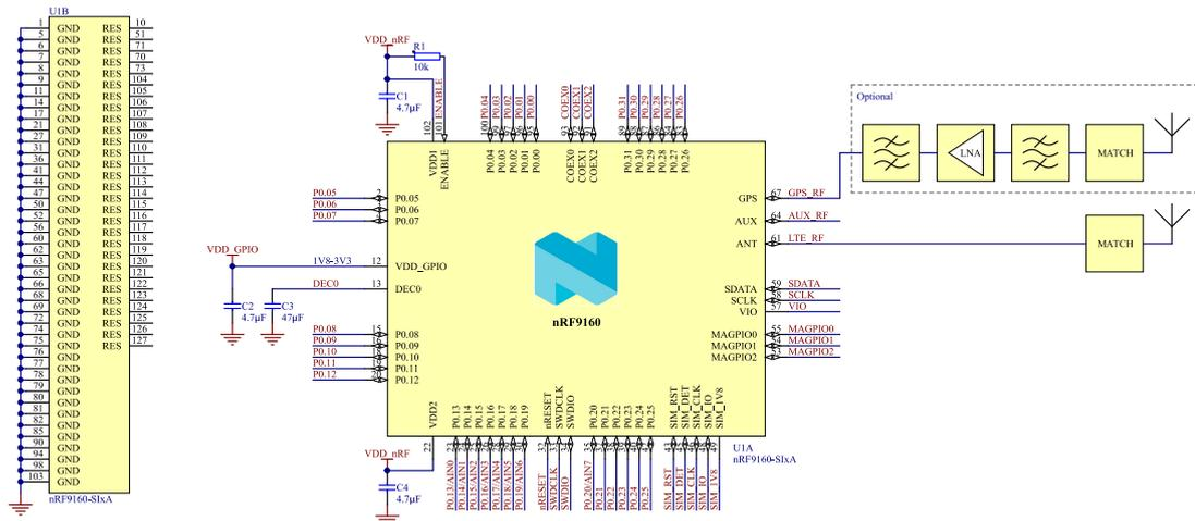
Figure 115: Schematic SixA with antenna details
