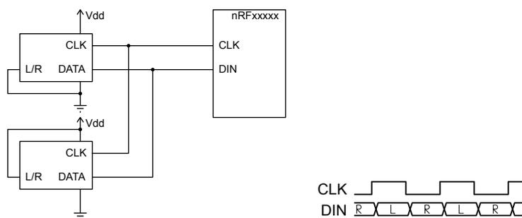
Figure 39: Example of two PDM microphones
