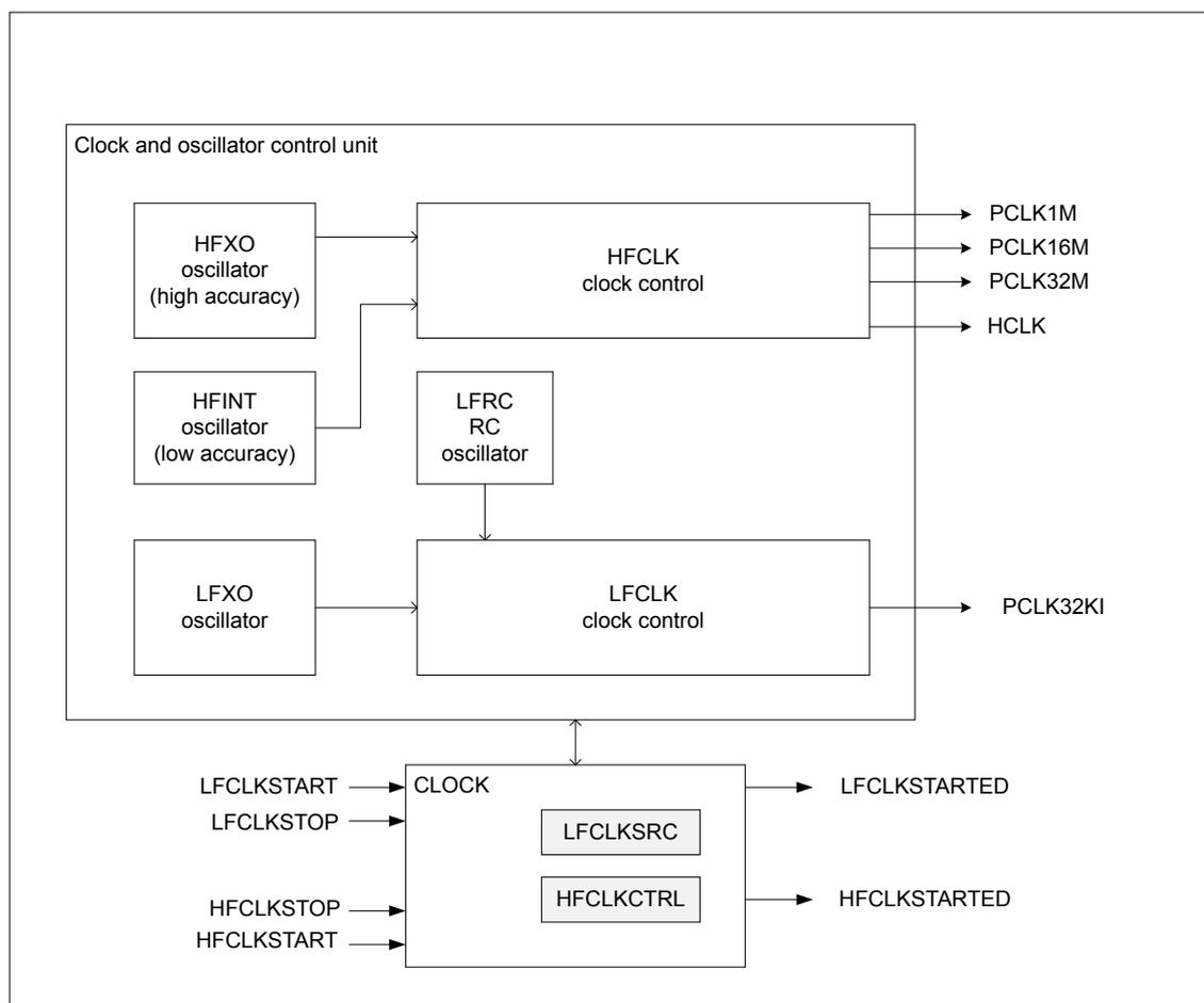
Figure 11: Clock and oscillator setup
