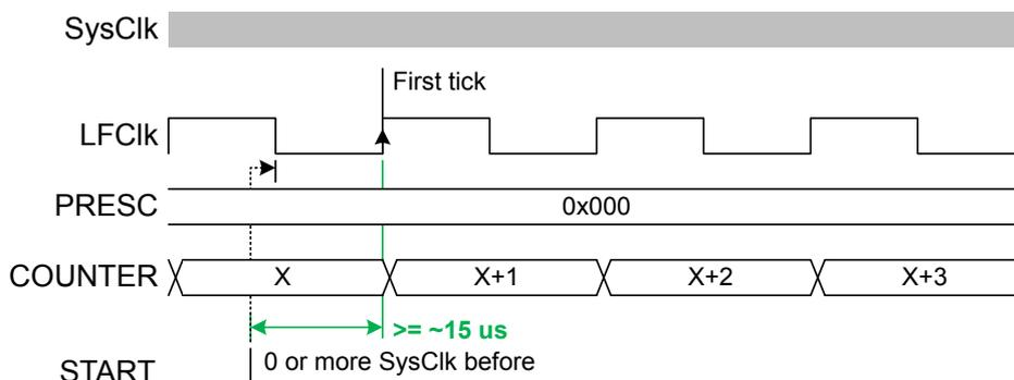
Figure 62: Timing diagram - JITTER\_START-
