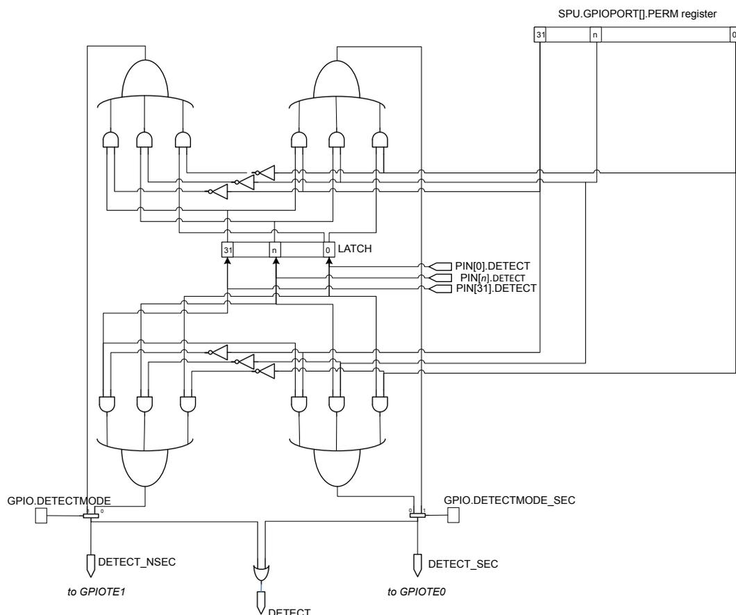
Figure 85: Principle of direct pin access
