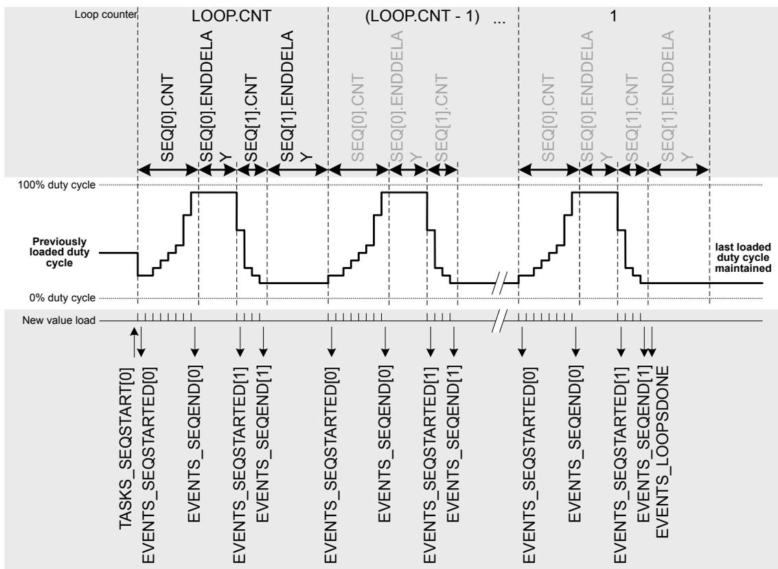
Figure 48: Complex sequence (LOOP.CNT>0) starting with SEQ[0]
