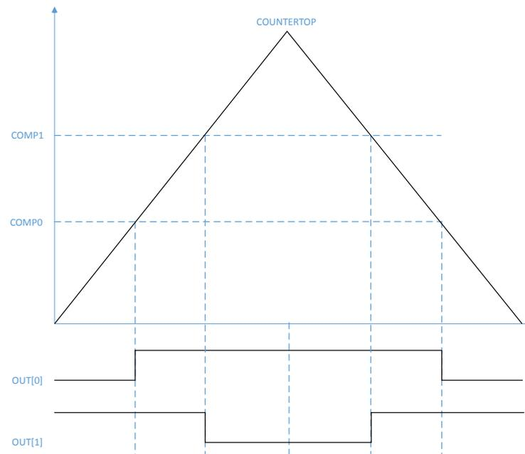
Figure 43: PWM counter in up-and-down mode example
