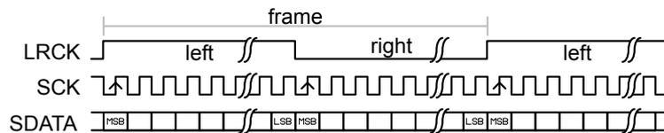
Figure 26: Aligned format. CONFIG.SWIDTH equalling half-frame size.
