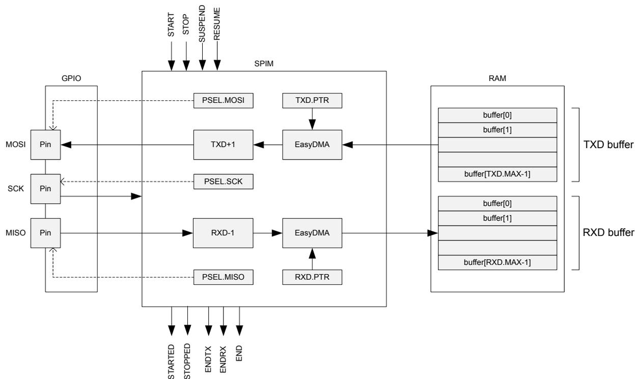
Figure 71: SPIM — SPI master with EasyDMA
