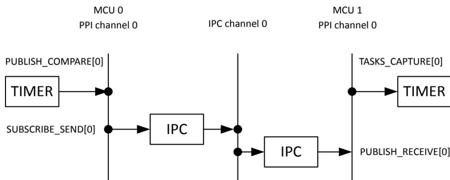
Figure 21: Example of PPI and IPC connections
