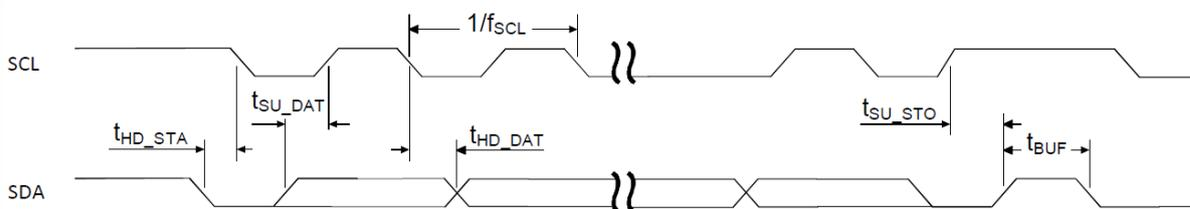
Figure 95: TWIM timing diagram, 1 byte transaction
