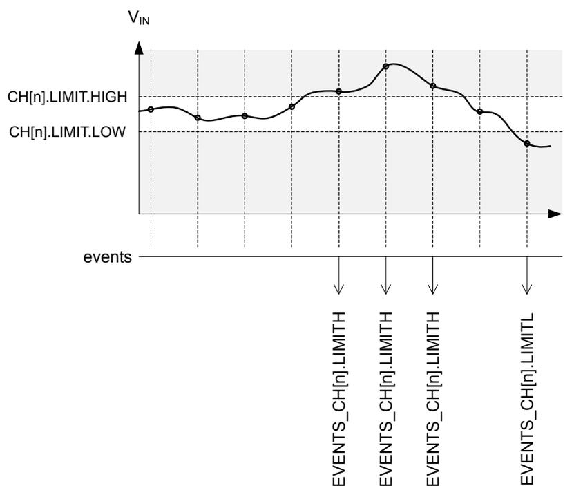
Figure 70: Example of limits monitoring on channel 'n'
