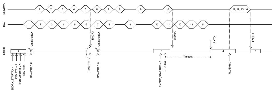
Figure 107: UARTe reception with forced stop via STOPRX
