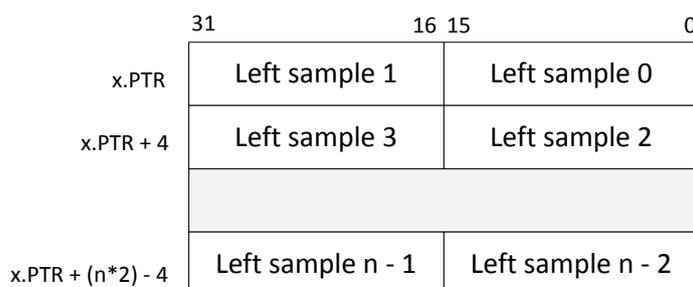
Figure 30: Memory mapping for 16 bit mono, left channel only. CONFIG.SWIDTH = 16Bit, CONFIG.CHANNELS = Left.
