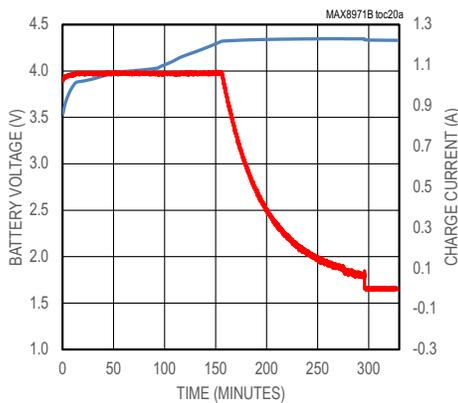
**CHARGE PROFILE FOR 1500mAh 4.2V BATTERY WITH 70mA CONSTANT LOAD CHARGED AT 0.6C**
