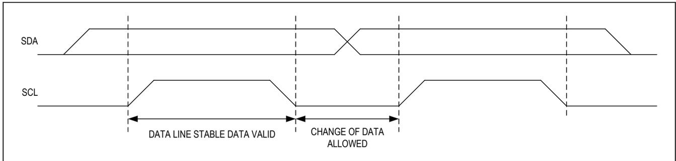
Figure 7. I<sup>2</sup>C Bit Transfer
