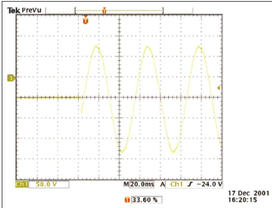
Figure 2. The ringer signal of a typical telephone exceeds 200V<sub>p-p</sub> (vertical scale is 50V/div).
