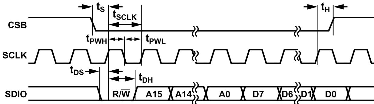
Figure 2. Timing Diagram for 3-Wire Write Operation
