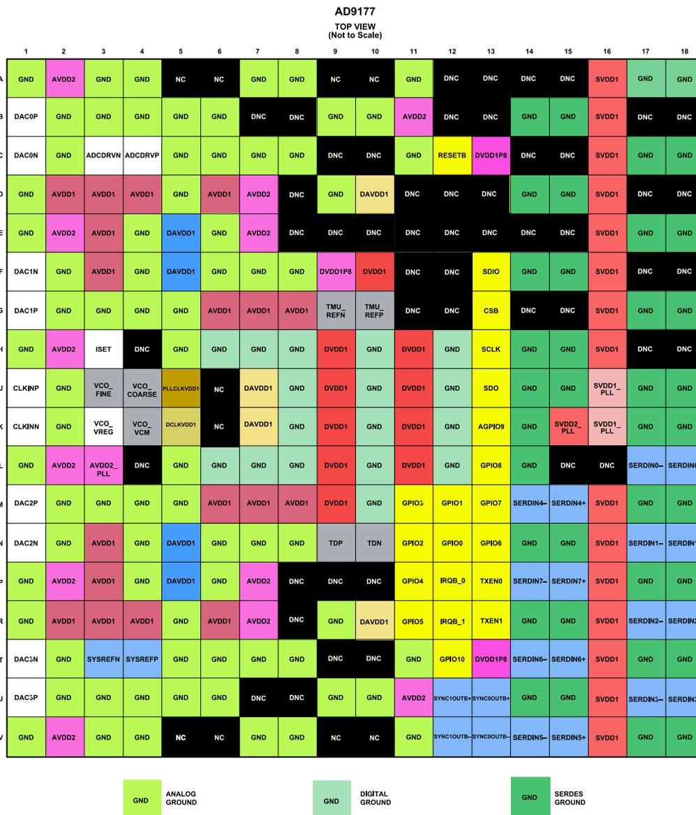
Figure 5. Pin Configuration
