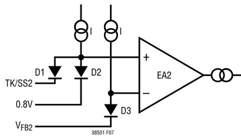
**Figure 7. Equivalent Input Circuit of Error Amplifier**
