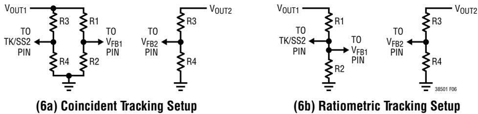
**Figure 6. Setup for Coincident and Ratiometric Tracking**
