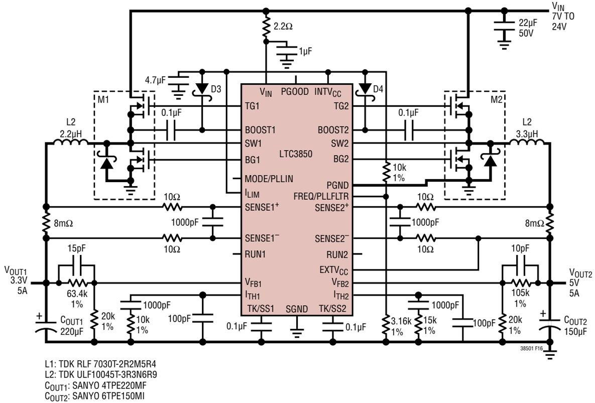
**Figure 16. 3.3V/5A, 5V/5A Converter Using Sense Resistors**
