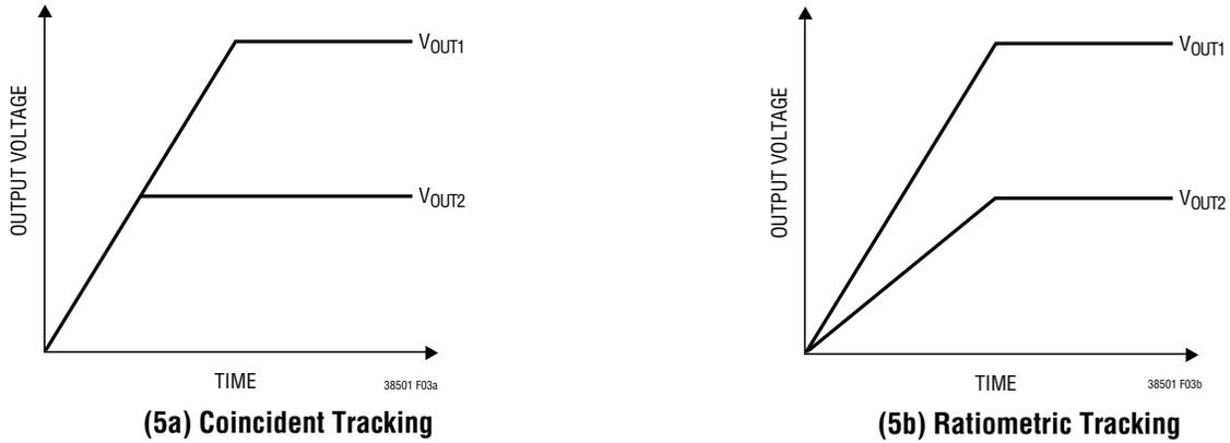
**Figure 5. Two Different Modes of Output Voltage Tracking**
