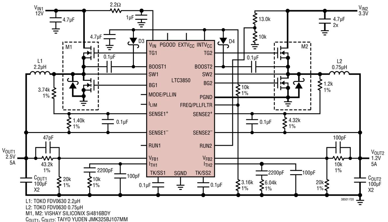
Figure 20. 2.5V/5A, 1.2V/5A Core-I/O Converter with Dual Inputs
