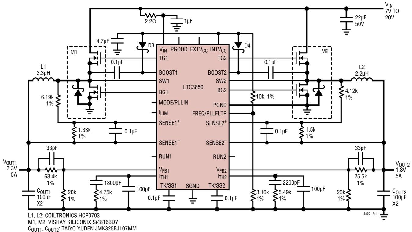
**Figure 14. High Efficiency Dual 500kHz 3.3V/1.8V Step-Down Converter**
