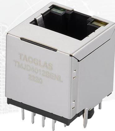
Featuring a popular footprint and compatible package to industry RJ45 Integrated Connectors standards, the Taoglas TMJD4012BENL is an RJ45 Integrated Connector 10/100Base-T Single Port and Vertical with shielded body and with a schematic that enables AutoMDIX feature.
