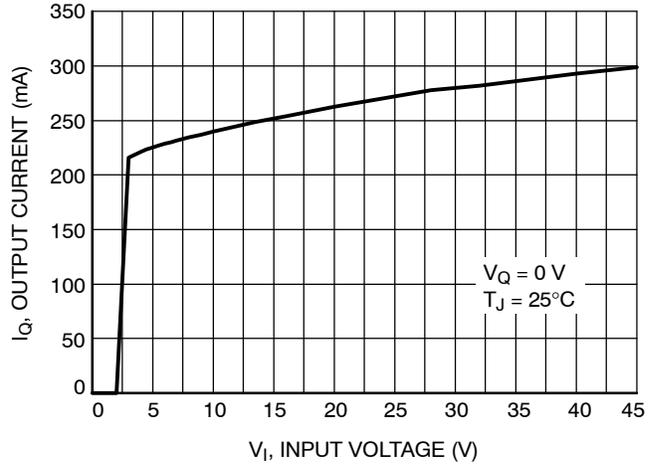
Figure 16. Maximum Output Current vs. Input Voltage
