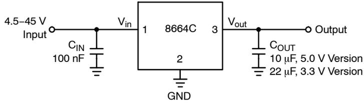
**Figure 3. Applications Circuit**
