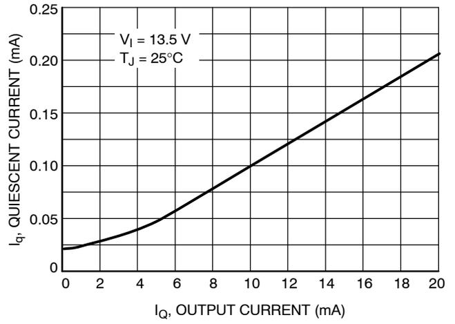
Figure 20. Quiescent Current vs. Output Current, (Low Load)
