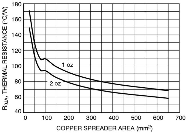
Figure 21. R<sub>θJA</sub> vs. Copper Spreader Area, SOT-223
