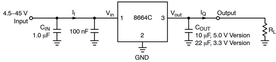
**Figure 2. Measurement Circuit**
