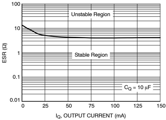
Figure 13. Output Stability with Output Capacitor ESR
