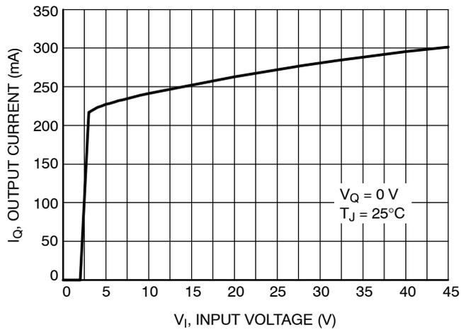
Figure 8. Maximum Output Current vs. Input Voltage
