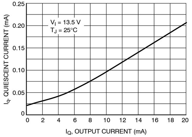
Figure 11. Quiescent Current vs. Output Current, (Low Load)
