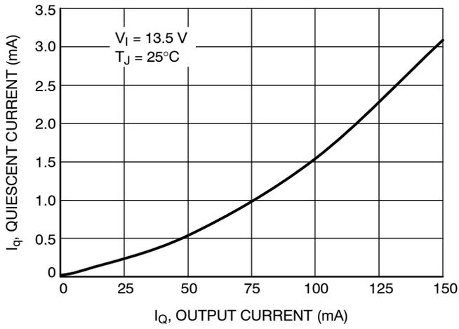
Figure 10. Quiescent Current vs. Output Current, (High Load)
