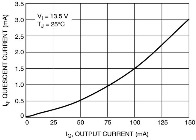
Figure 19. Quiescent Current vs. Output Current, (High Load)
