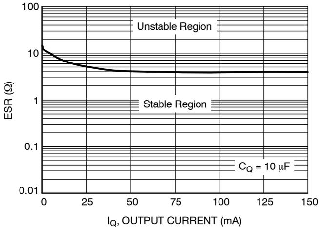
Figure 4. Output Stability with Output Capacitor ESR
