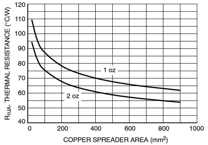
Figure 22. R<sub>θJA</sub> vs. Copper Spreader Area, DPAK
