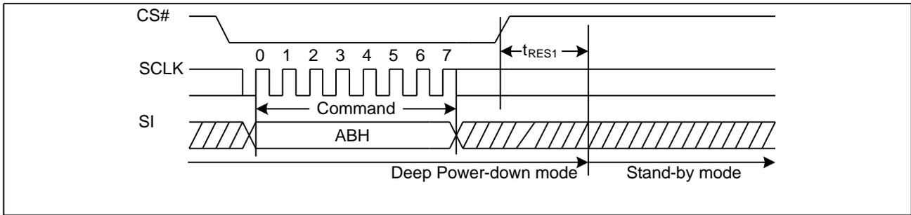
Figure 24. Release Power-Down/Read Device ID Sequence Diagram
