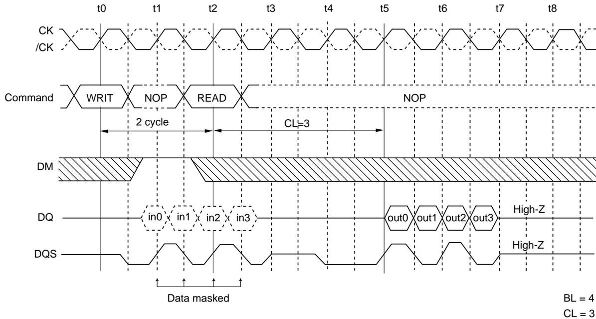
[WRITE to READ delay = 2 clock cycle]
