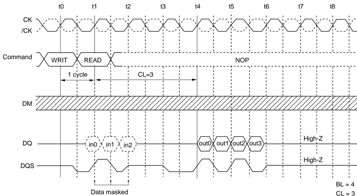
[WRITE to READ delay = 1 clock cycle]
