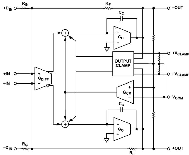
Figure 99. ADA4945-1 Architectural Block Diagram
