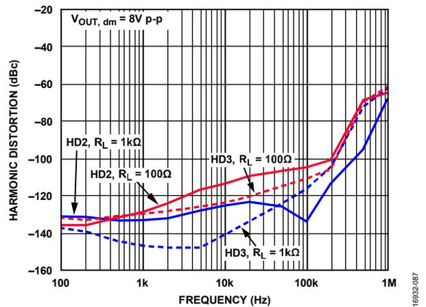
Figure 65. Harmonic Distortion vs. Frequency for Various Loads
