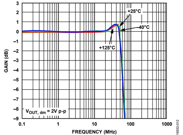
Figure 9. Large Signal Frequency Response for Various Temperatures
