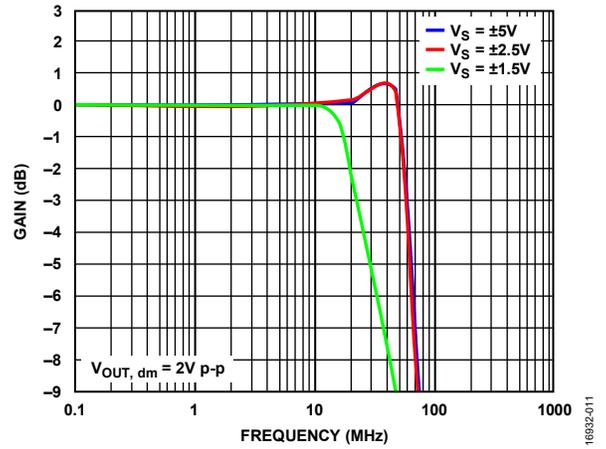
Figure 8. Large Signal Frequency Response for Various Supplies
