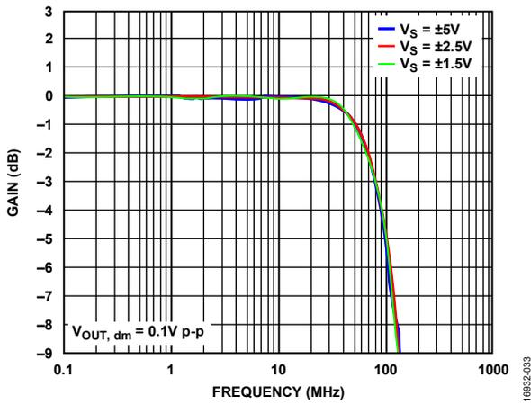
Figure 50. Small Signal Frequency Response for Various Supplies
