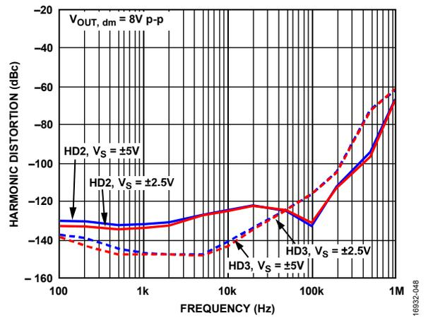
Figure 66. Harmonic Distortion vs. Frequency for Various Supplies
