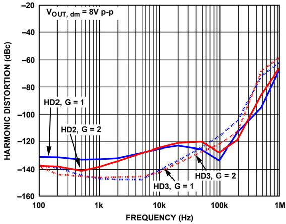
Figure 67. Harmonic Distortion vs. Frequency for Various Gains
