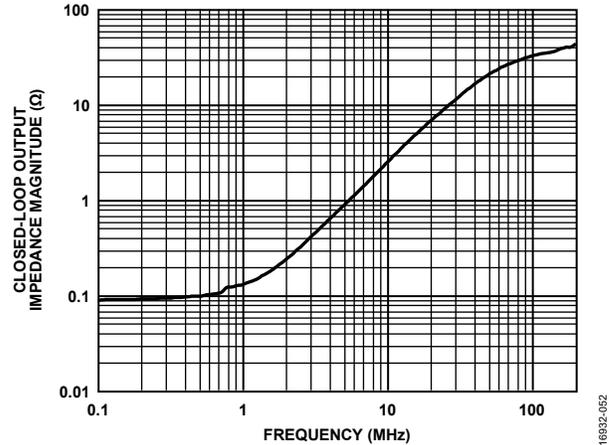
Figure 82. Closed-Loop Output Impedance Magnitude vs. Frequency,  $G = 1$
