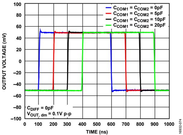
Figure 87. Small Signal Transient Response for Various Capacitive Loads,  $V_S = 3\text{ V}$
