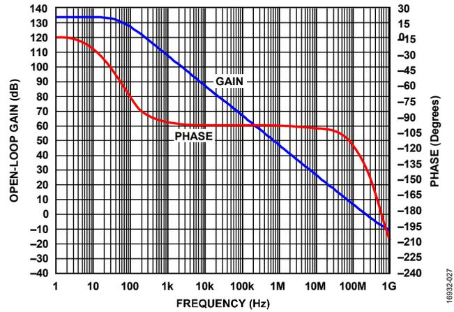
Figure 31. Open-Loop Gain and Phase vs. Frequency
