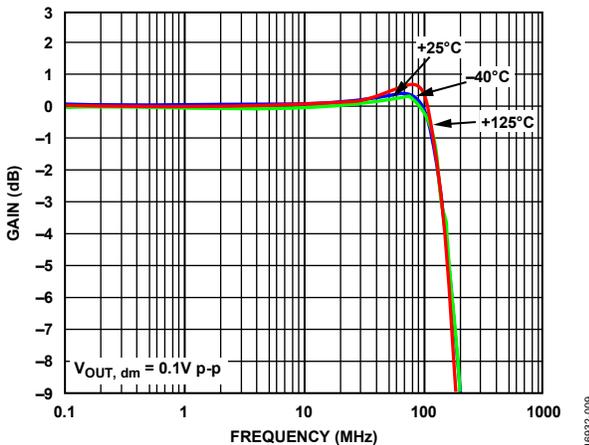
Figure 6. Small Signal Frequency Response for Various Temperatures
