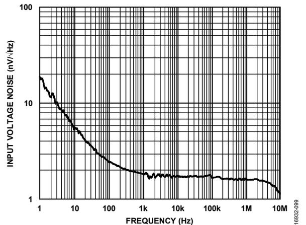
Figure 33. Voltage Noise Spectral Density, Referred to Input
