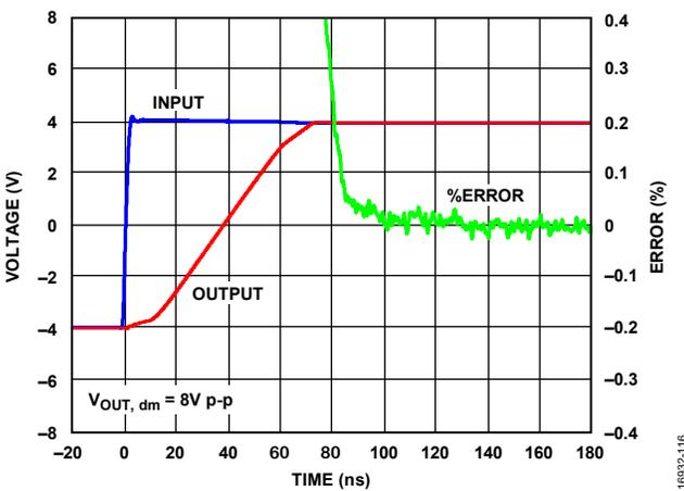
Figure 81. 0.1% Settling Time
