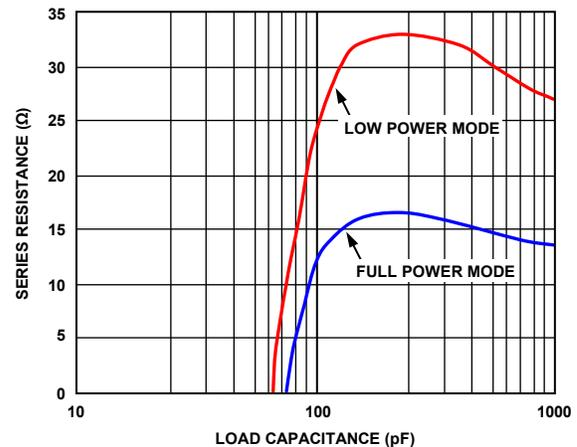
Figure 111. Series Resistance vs. Load Capacitance
