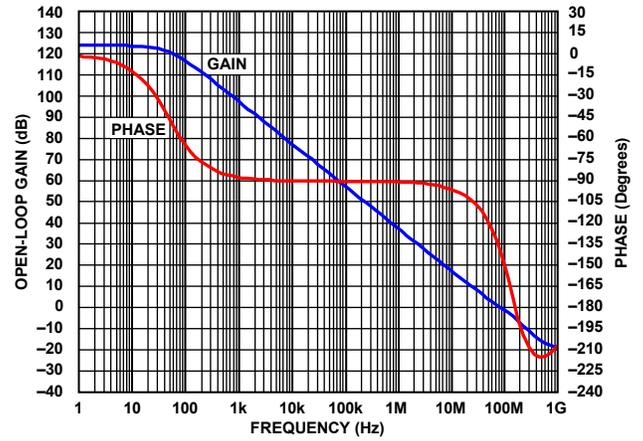
Figure 76. Open-Loop Gain and Phase vs. Frequency
