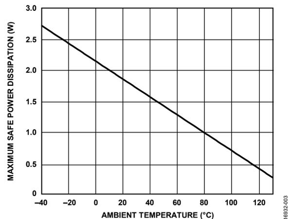
Figure 2. Maximum Safe Power Dissipation vs. Ambient Temperature
