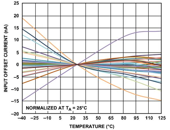
Figure 64. Input Offset Current vs. Temperature for 30 Devices
