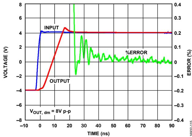
Figure 36. 0.1% Settling Time
