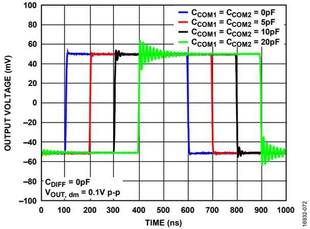
Figure 85. Small Signal Transient Response for Various Capacitive Loads,  $V_S = 10\text{ V}$
