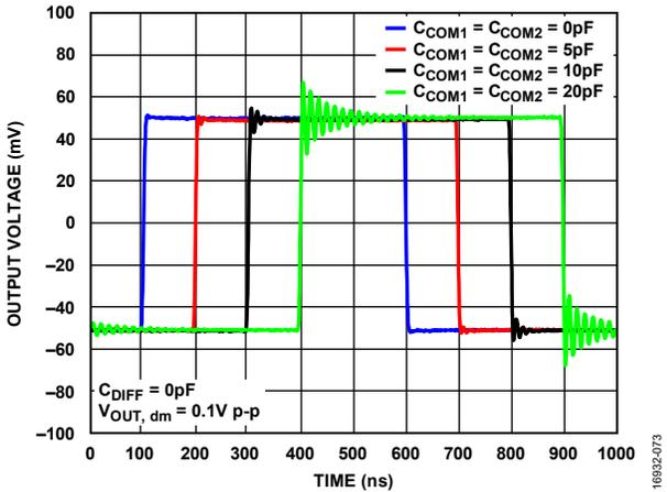
Figure 86. Small Signal Transient Response for Various Capacitive Loads,  $V_S = 5\text{ V}$
