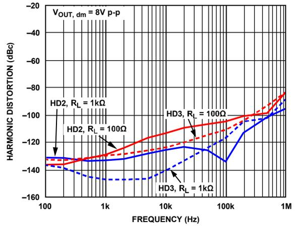
Figure 20. Harmonic Distortion vs. Frequency for Various Loads
