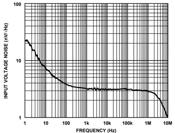
Figure 78. Voltage Noise Spectral Density, Referred to Input
