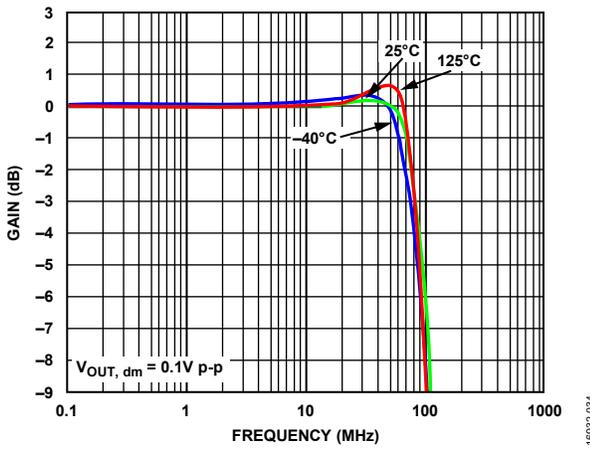
Figure 51. Small Signal Frequency Response for Various Temperatures
