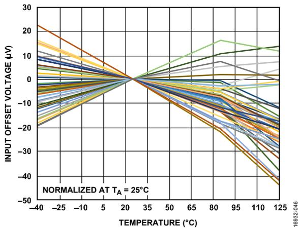
Figure 63. Input Offset Voltage vs. Temperature for 50 Devices
