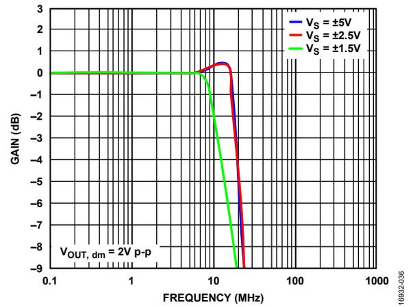
Figure 53. Large Signal Frequency Response for Various Supplies
