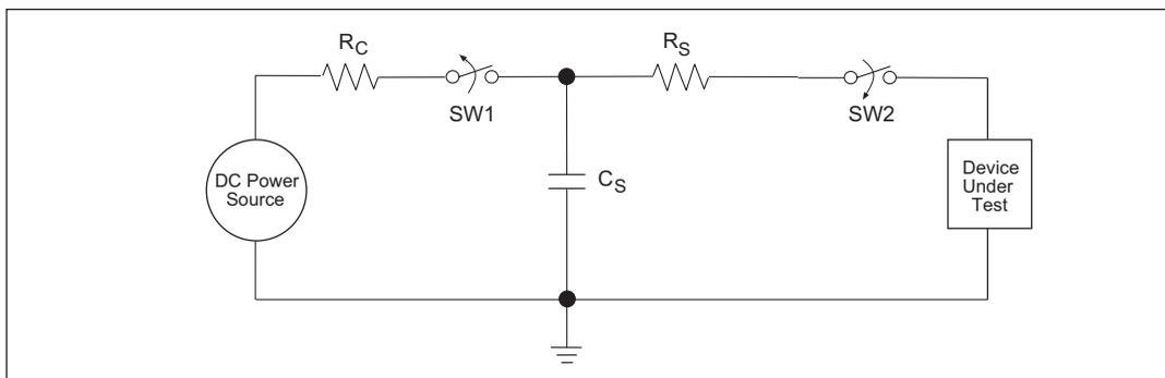
Figure 19. ESD Test Circuit for Human Body Model
