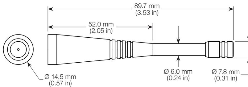
Figure 7. CW LTE Band 20 Antenna Dimensions
