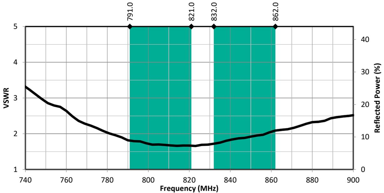
Figure2. CW LTE Band 20 Antenna Full Bandwidth VSWR
