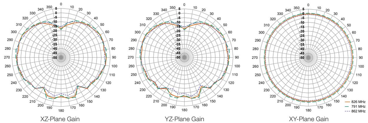
Figure9. Radiation Patterns for CW LTE Band 20 Antenna
