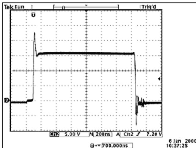
Figure 7. Waveform after output diode.
