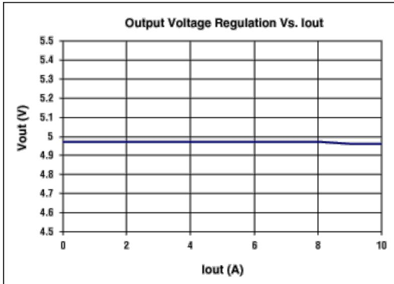
Figure 10. Output-voltage regulation.
