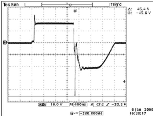
Figure 4. Waveform at transformer secondary.
