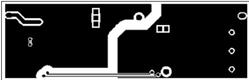
Figure 13. Bottom side copper tracks of the FWD0510 power supply.
