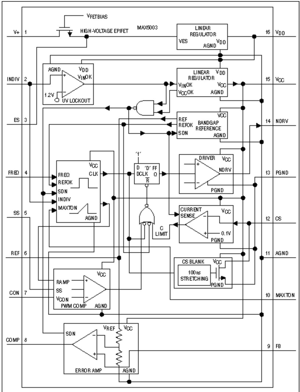
Figure 3. MAX5003 block diagram.
