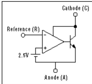
Figure 6. Simplified block diagram of the shunt regulator.
