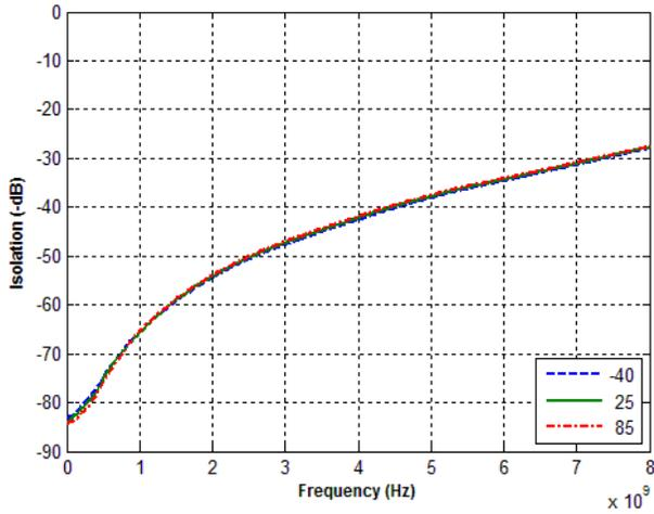
**Figure 17. Isolation vs.  $V_{DD}$  (RFC-RFX)**
