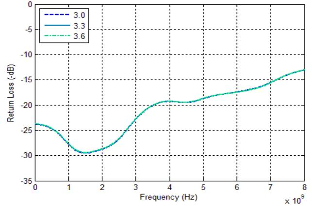
**Figure 10. Active Port Return Loss vs. Temp**
