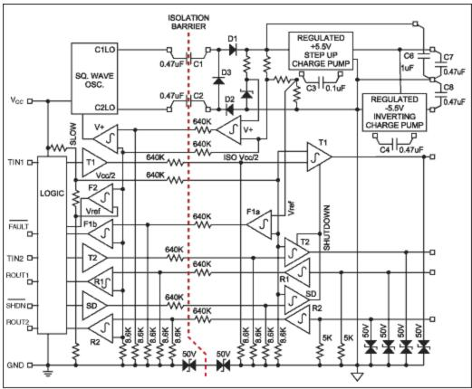
Figure 1. MAX3250 functional block diagram.
