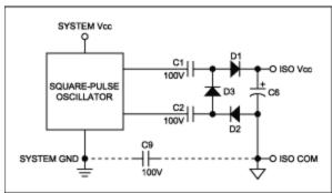
Figure 4. Capacitor-coupled isolated supply.
