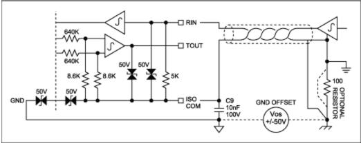
Figure 5. MAX3250 line interface circuitry with shielded line.
