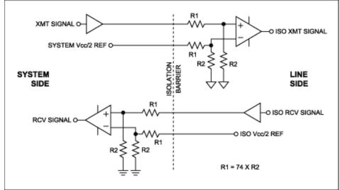
Figure 3. Resistive isolation technique.
