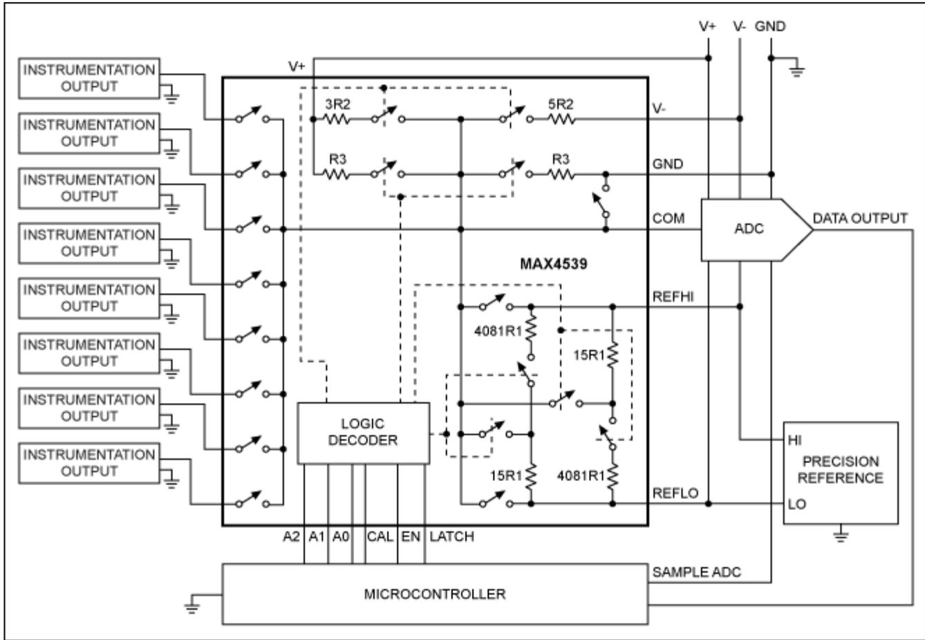
Figure 1. The MAX4539 cal-mux simplifies calibration of a multi-channel industrial control system.
