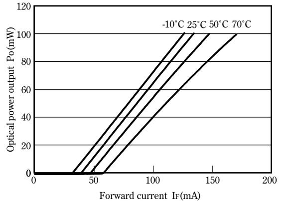
Case temperature dependence of threshold current [CW]
