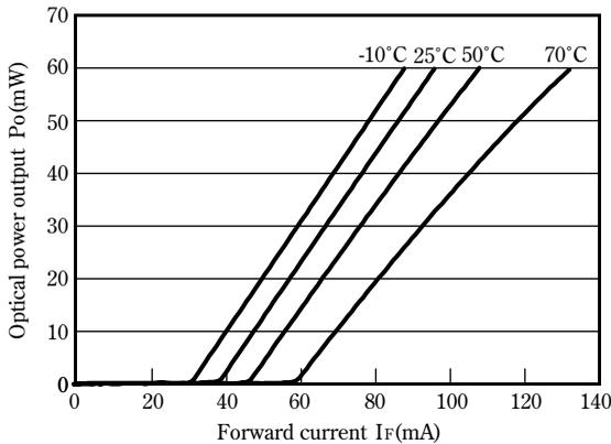
Optical power output - Forward current [Pulse]
