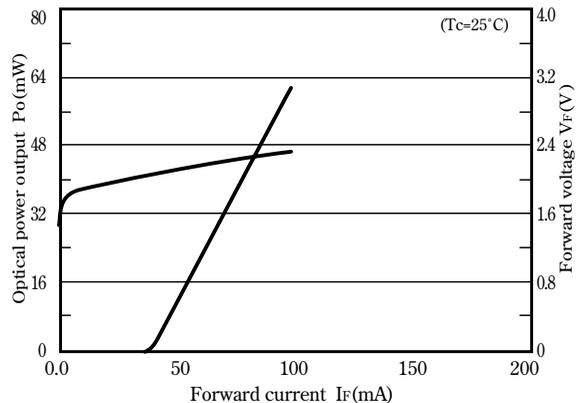
Forward voltage - Forward current [Pulse]
