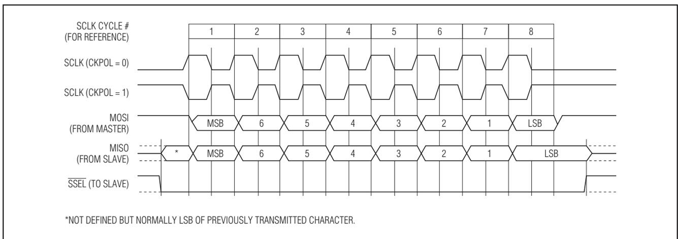
Figure 4b. SPI Interface Timing (CKPHA = 1)
