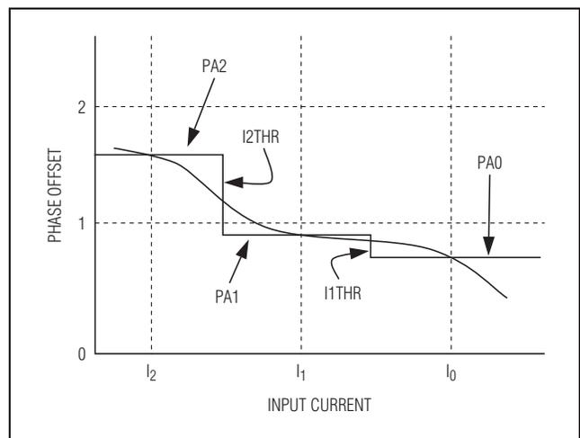
Figure 16. Phase Offset vs. Input Current Calibration
