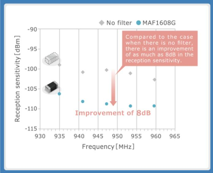
Figure 5: Result of insertion of MAF1608G into the speaker line (improvement in reception sensitivity) (2)
