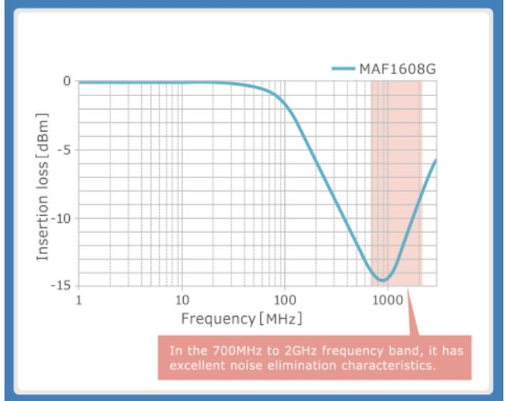
Thus, it can be seen that the application of MAF1608G to audio lines is extremely effective as a solution to the problem of degradation of reception sensitivity in smartphones. But what about the problem of voice distortion caused by insertion?
