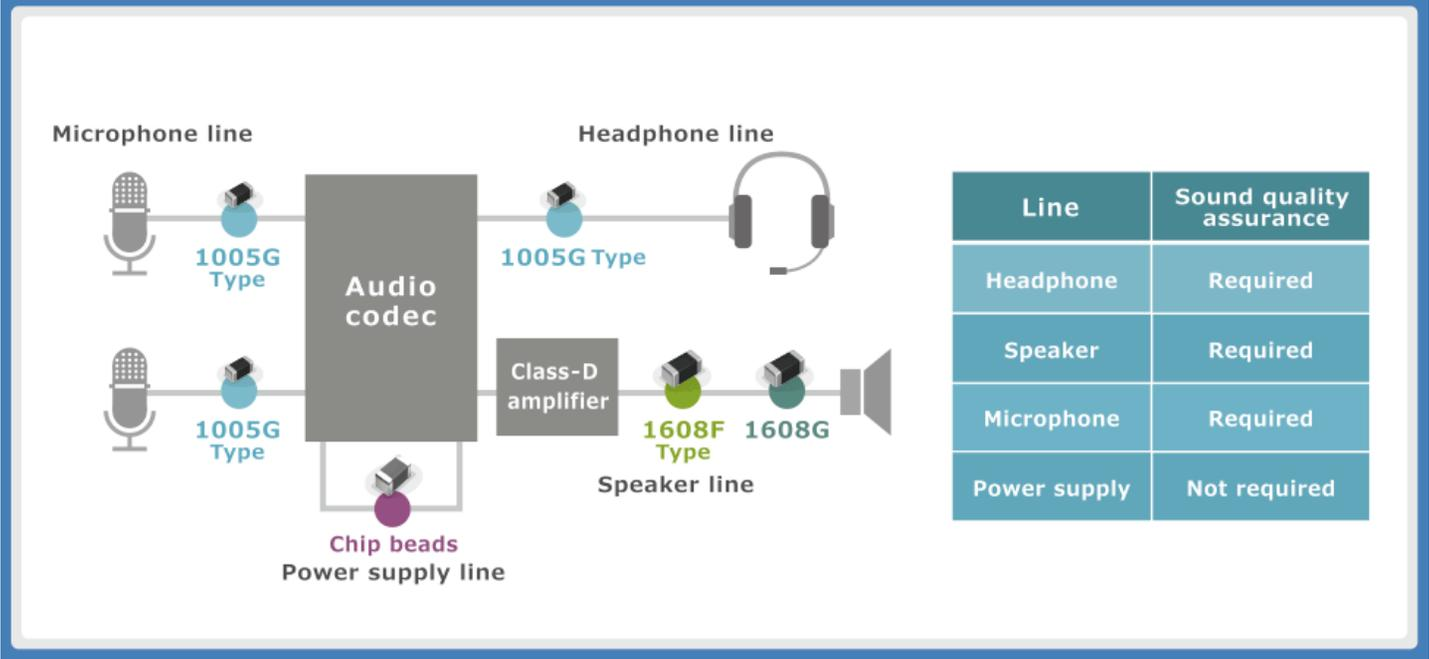
《Main features and applications of the MAF series of noise suppression filters for audio lines》
