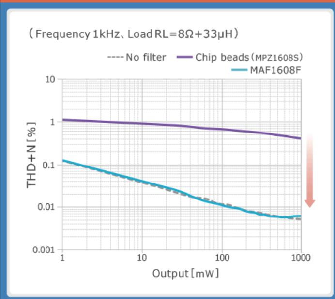
**Figure 8: Result of insertion of MAF1608F into the speaker line (2) Effect of suppression of noise emission in Class-D amplifiers by using MAF1608F**
