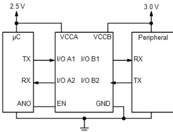
**Figure 8. Application Example for A < B**
