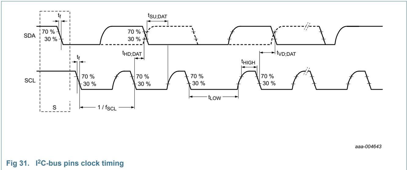
Fig 31. I<sup>2</sup>C-bus pins clock timing
