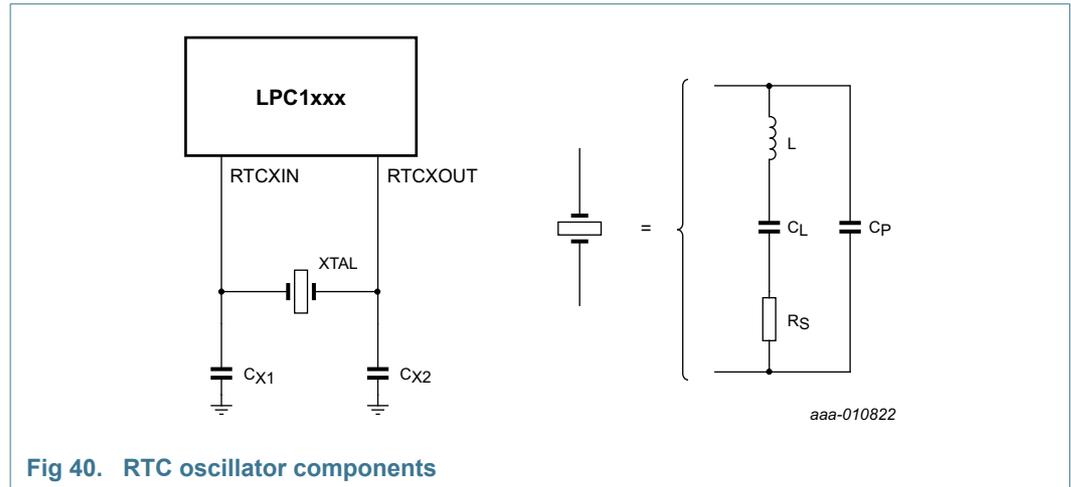
Fig 40. RTC oscillator components
