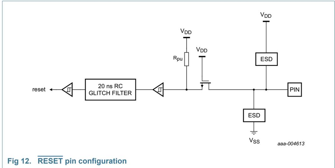
Fig 12. RESET pin configuration
