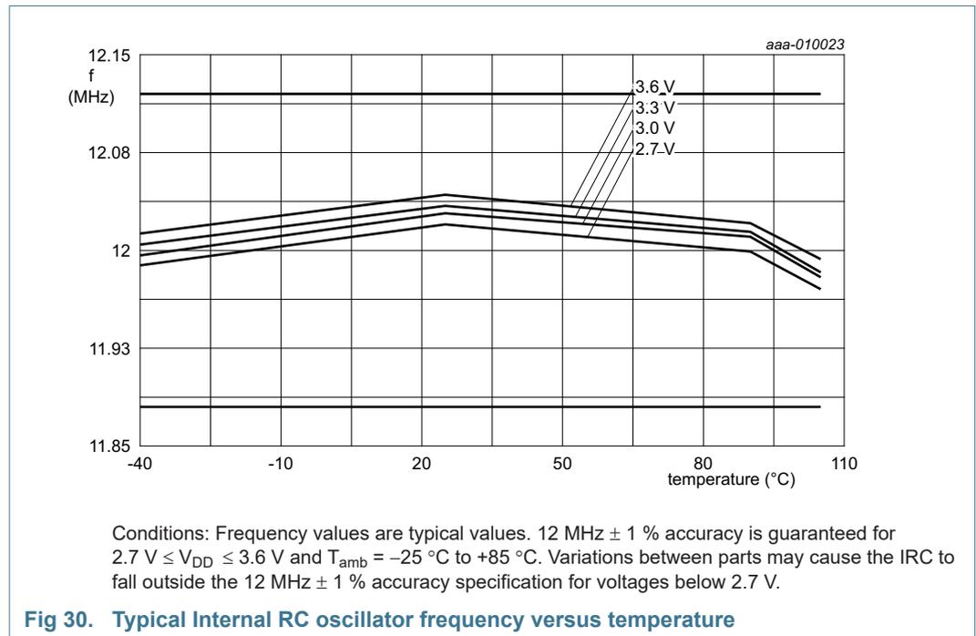
Fig 30. Typical Internal RC oscillator frequency versus temperature
