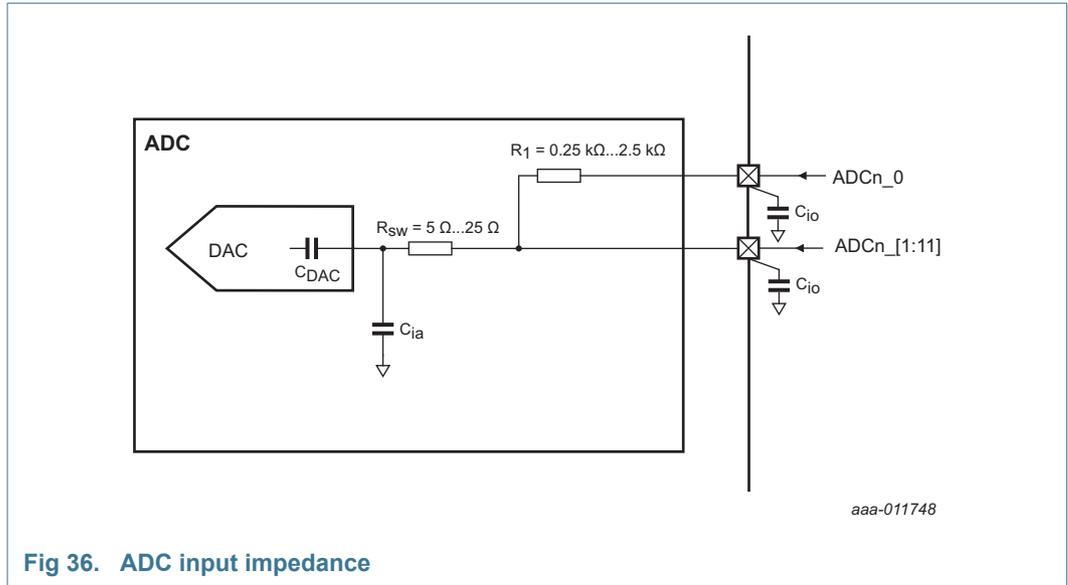
Fig 36. ADC input impedance
