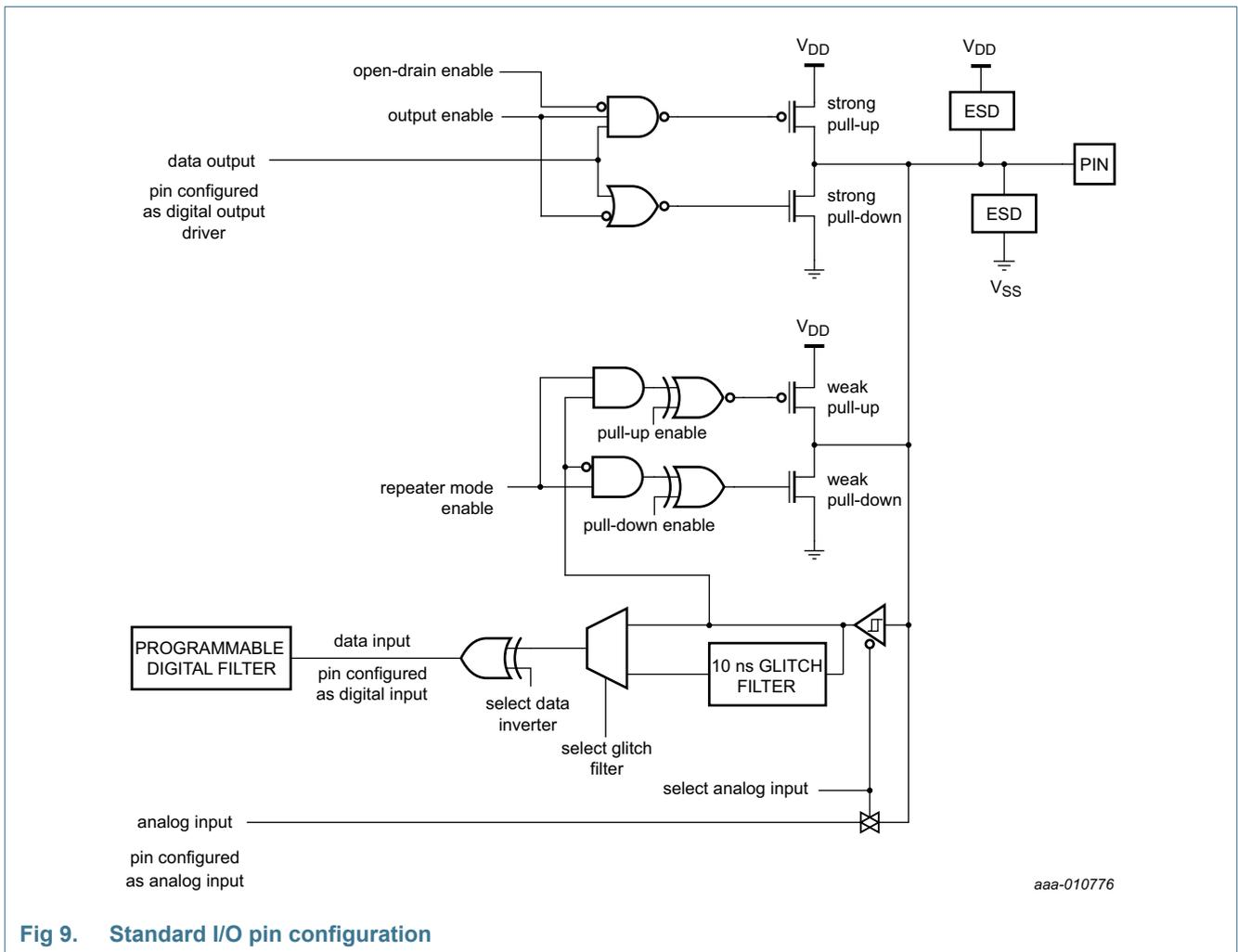
Fig 9. Standard I/O pin configuration
