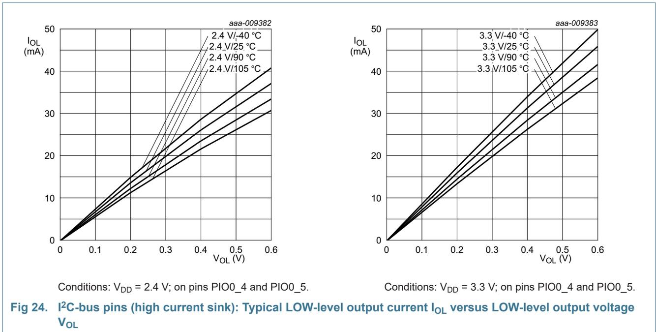
Fig 24. I<sup>2</sup>C-bus pins (high current sink): Typical LOW-level output current  $I_{OL}$  versus LOW-level output voltage  $V_{OL}$
