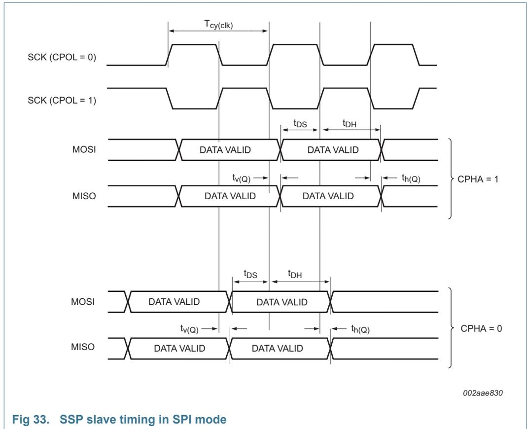
Fig 33. SSP slave timing in SPI mode
