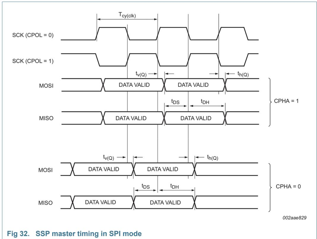
Fig 32. SSP master timing in SPI mode
