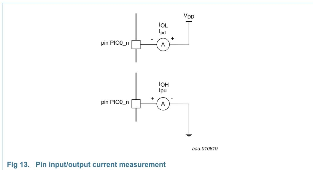
Fig 13. Pin input/output current measurement
