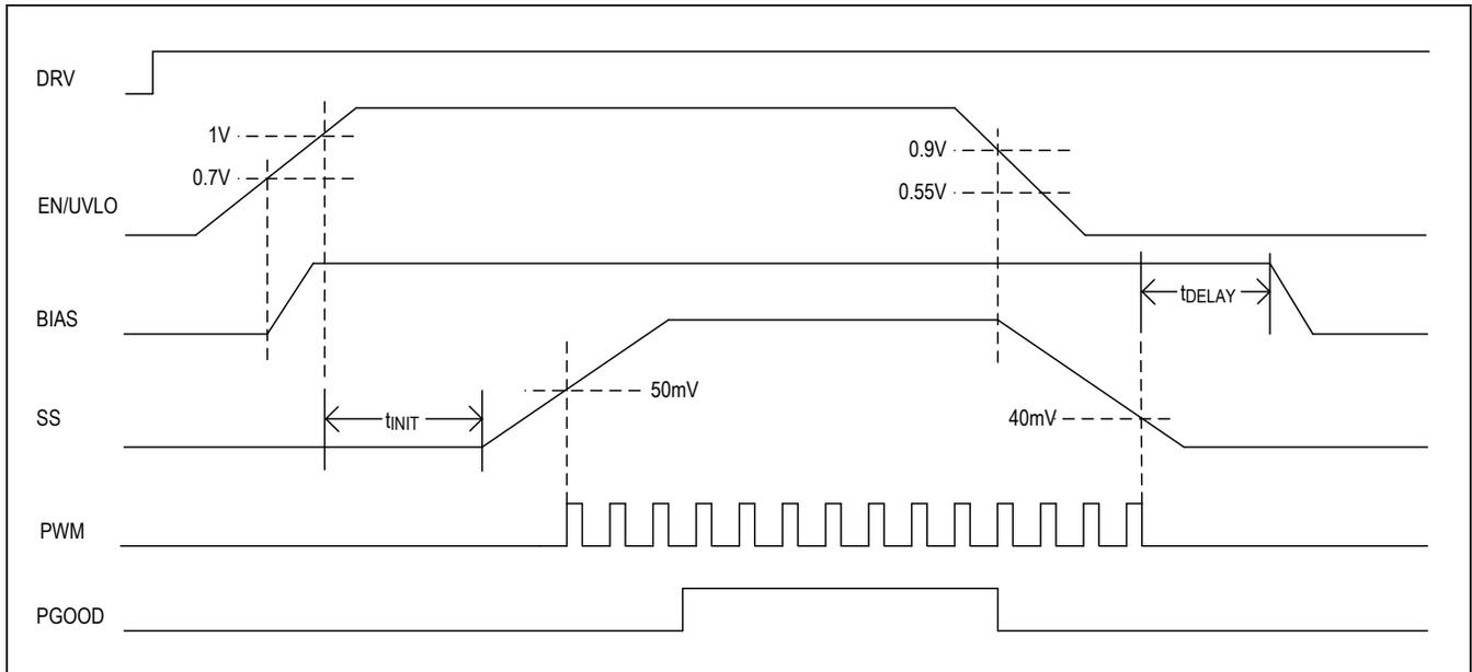
Figure 5. Soft-Start and Shutdown Sequence with EN/UVLO
