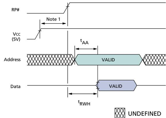
**NOTE:** 1.  $V_{CC}$  must be within the valid operating range before RP# goes HIGH.
