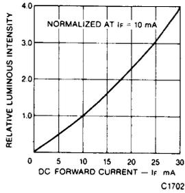
Fig. 2. Relative Luminous Intensity vs. DC Forward Current
