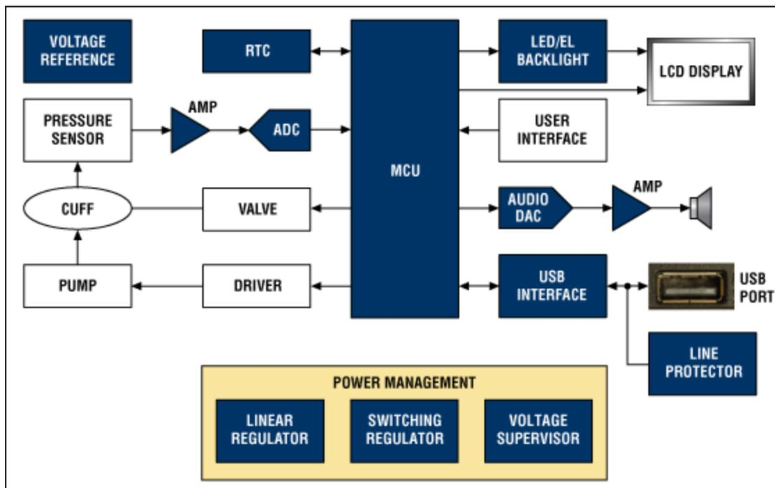
Functional block diagram of a blood pressure monitor that includes an advanced voice indicator. For a list of Maxim's recommended solutions for blood pressure monitor designs, please go to: [www.maximintegrated.com/bloodpressure](http://www.maximintegrated.com/bloodpressure).
