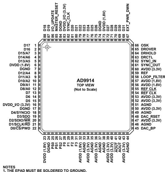
Figure 3. Pin Configuration
