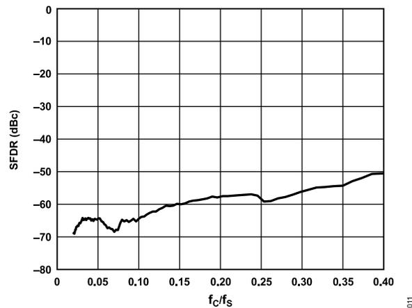
Figure 11. Wideband SFDR vs. Normalized  $f_{OUT}$ , SYSCLK = 3.5 GHz
