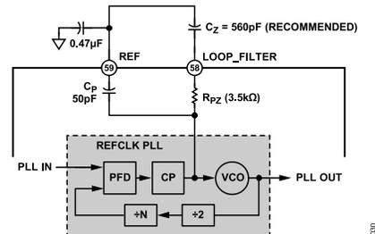
Figure 35. REF CLK PLL External Loop Filter
