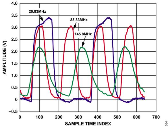
Figure 22. SYNC\_CLK Amplitude at Various Frequencies ( $f_{\text{SYSCLK}}/24$ ), Measured at the SYNC\_CLK Pin Using an Active Probe (1 GHz Bandwidth, 1  $\Omega$ , 1 pF) with the SYNC\_CLK Pin Loaded by a 1-inch PCB Trace Connected to an Open SMA Connector
