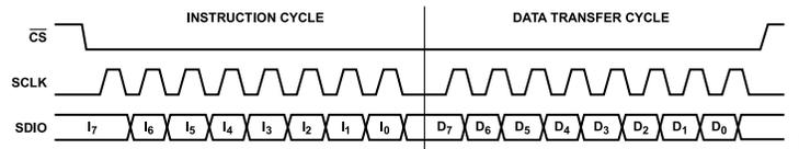
Figure 43. Serial Port Write Timing, Clock Stall Low
