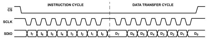
Figure 45. Serial Port Write Timing, Clock Stall High
