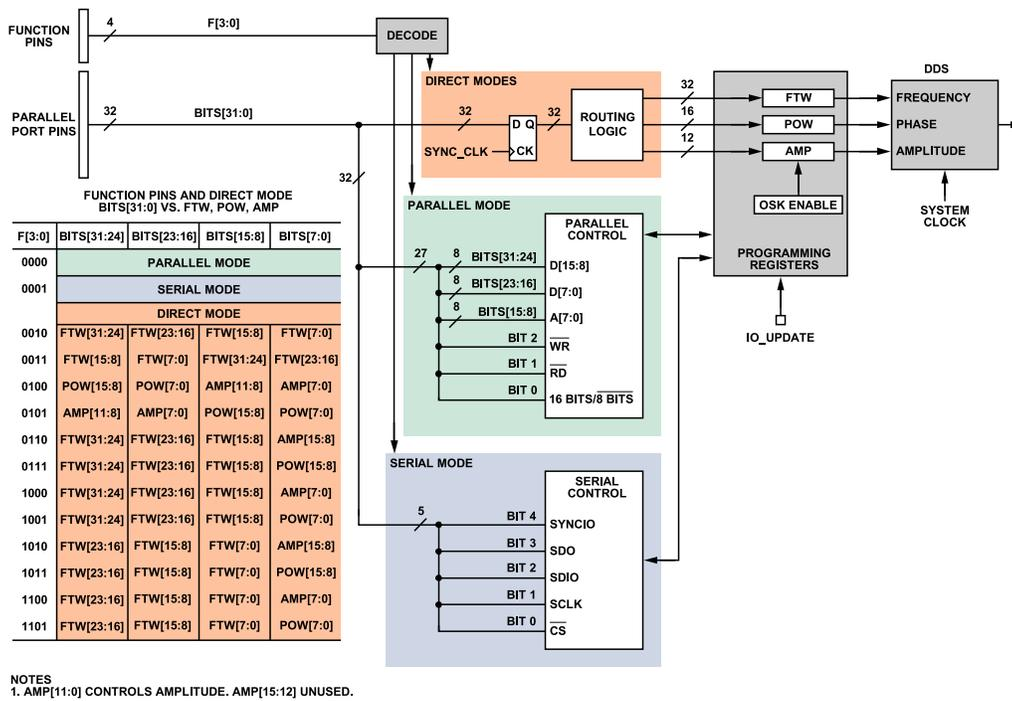
Figure 42. Parallel Port Block Diagram
