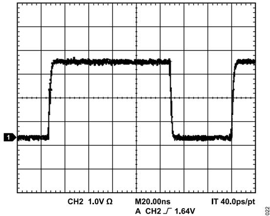
Figure 23. SYNC\_OUT ( $f_{\text{SYSCLK}}/384$ )
