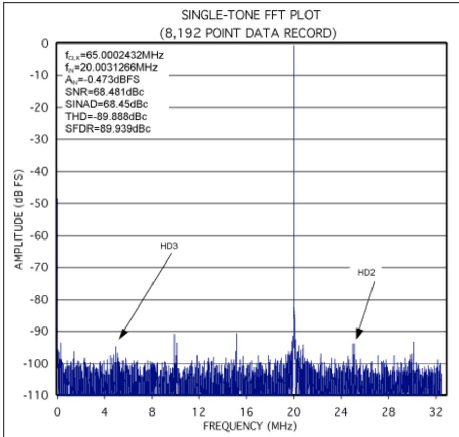
Figure 2. Coherently sampled FFT from the MAX1211EVKIT.
