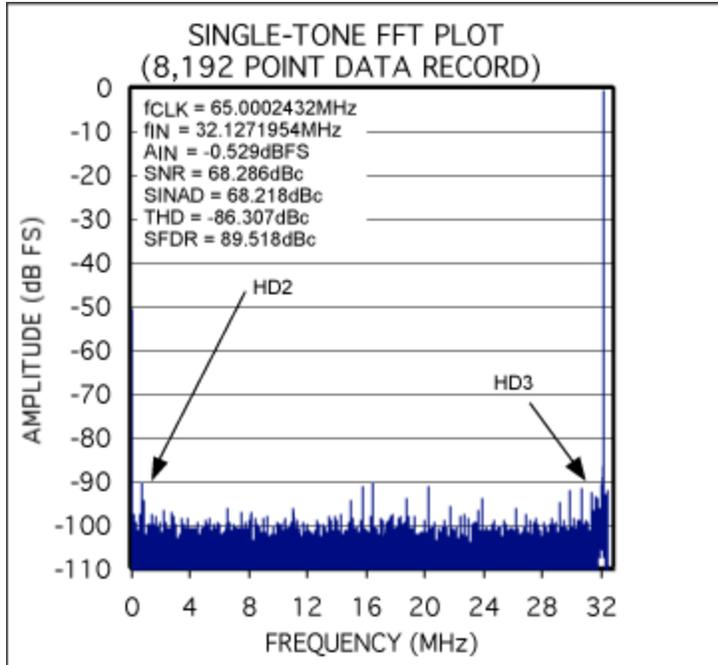
Figure 3. Coherently sampled FFT from the MAX1211EVKIT.
