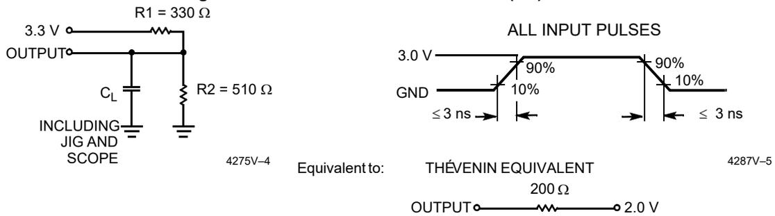
Figure 5. AC Test Loads and Waveforms (-10)
